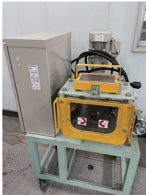
図 14 炭酸化処理に用いたバッチ式パグミルミキサー Batch-type pugmill mixer used for carbonation experiments A laboratory-scale batch-type pugmill mixer manufactured by Shin-Nichinan Co., Ltd. The mixer has a nominal vessel capacity of 6 L and features a twin-shaft paddle configuration designed to generate compressive forces between paddles.
