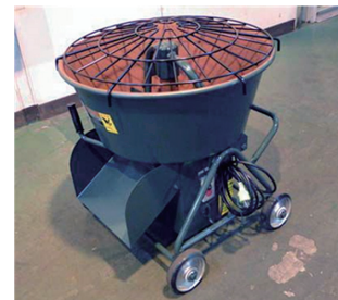
図10 炭酸化処理に用いたモルタルミキサー Mortar mixer used for the carbonation treatment of steel-making slag The mixer (Model PM-15N, Mazella Co., Ltd.) was operated at 48rpm, with water added at 10mass% of the slag and CO 2 supplied at 0.018mol min/kg-slag. During operation, the top of the mixer was covered with a plastic sheet to prevent intrusion of outside air. The internal CO 2 concentration increased gradually after injection and stabilized at 90-95vol% after 30minutes.
