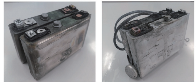
図 7 類焼試験後の電池外観 Appearances of lithium-ion batteries after thermal runaway propagation test
