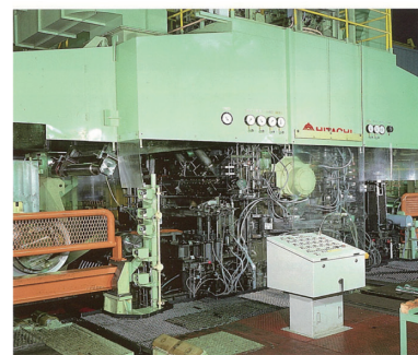
(a) Precision cold-rolling mill for finish rolling of thin steel sheets
