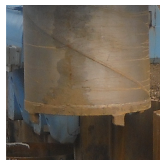
写真2 鋼管杭の先端ビット Bit that was attached to the tip of steel pipe pile
