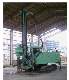
(b) Small-diameter pile
