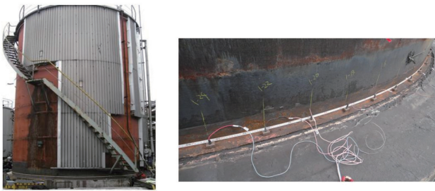
写真5 被検査体および直流電位差法による計測状況 Inspected object and outline of inspection by direct current potential different method
