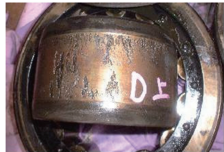
写真1 開放点検軸受 Overhaul inspection of defective bearing
