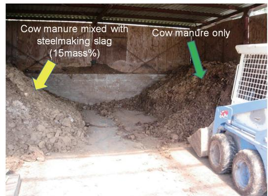
図8 堆肥化試験の様子 Composting of cow manure
