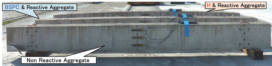
写真1 ASRを促進させたPC梁試験体の暴露状況 Exposure of the PC beam specimen which accelerated ASR
