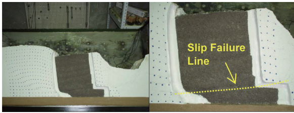
写真2 遠心力模型実験後の地盤の破壊、変形状態 State of failure and deformation of ground after centrifuge model test
