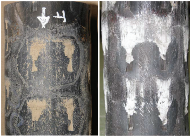
図13 押し抜き試験後の窪み表面 (左：ソイルセメント (2MPa) 右：モルタル (36MPa)) Observation on the outer surface of test pipes after bonding tests (left: soil-cement of 2 MPa; right: mortar of 36 MPa)
