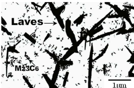
写真1 750℃、3000h時効材の抽出レプリカ組織 TEM microstructure of extracted replica of HR6W aged at 750℃ for 3000h
