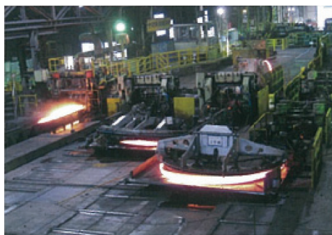
図3 ステンレス形鋼用熱間圧延機 Hot rolling mill for rolled shape stainless steel
