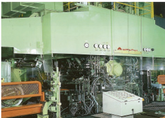
図6 ステンレス鋼仕上げ圧延用精密圧延機 Precision rolling mill for finish rolling of thin stainless steel sheets and coils
