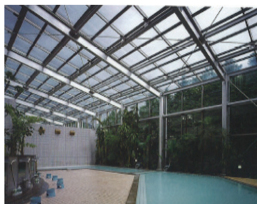
図9 ステンレス形鋼の使用例 (ホテル霧島キャッスル) Example of an application of stainless shaped rolled products, courtesy to Hotel Kirishima Castle
