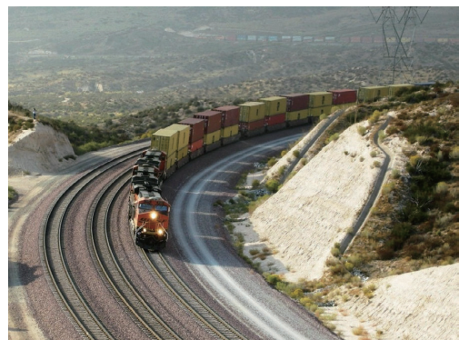
写真1 海外の貨物鉄道における重載化の事例 Example of increase of superimposed load on an overseas freight railway
