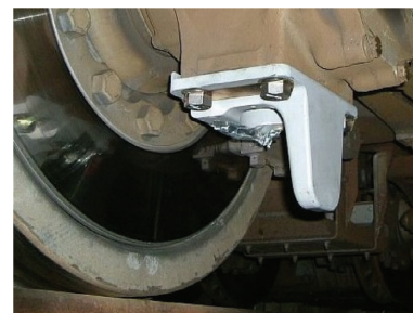
図12 逸脱防止L型ガイド L-shaped guide to prevent deviation from rails
