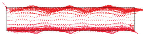
図7 EMSによる溶鋼内電磁力分布(コア高さ中心) Lorentz force distribution in the molten steel at middle-height of the EMS core
