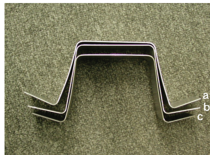
a: Aluminum alloy in warm forming at 10kN in BHF b: Aluminum alloy in warm forming at 150kN in BHF c: Steel in cold forming at 10kN in BHF
