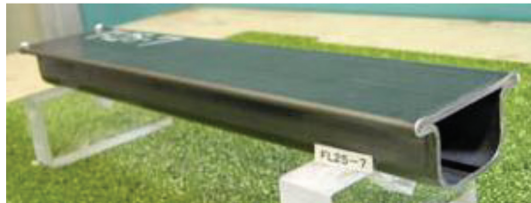
(a) Formed sample by hydroforming with flat seal technology
