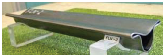
(b) Formed sample without internal pressure
