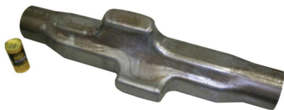
図5 直角方向に二枝張出し加工した例 15) Forming samples with two branches with right angle each other
