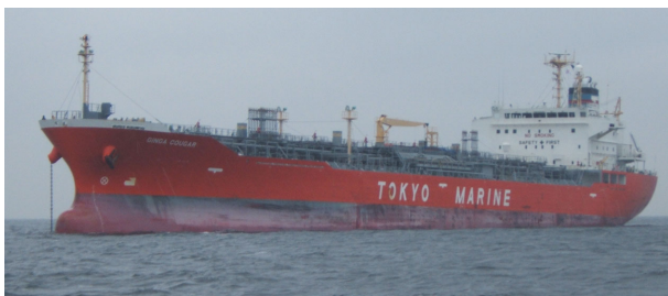
図6 NSSC 260A鋼を適用したケミカルタンカー Chemical tanker to which NSSC 260A stainless steel was applied
