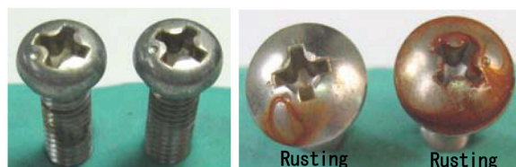
(a) Proper passivation (Non rust) (b) Improper passivation (Rusting)
