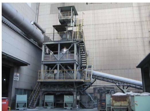
図5 破碎・粉砕処理装置外観写真 Photograph of crushing and milling equipment
