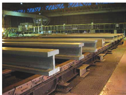
写真11 高機能極厚H形鋼 High performance extra-heavy [giant] H shape
