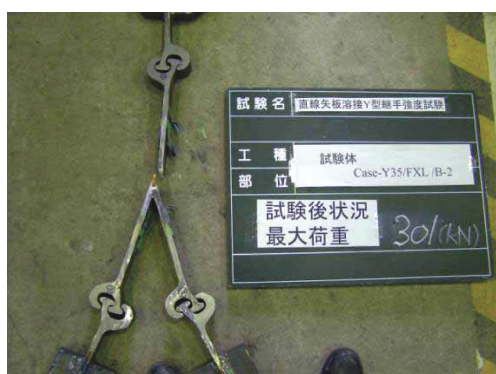
写真10 鋼矢板セル接合部y型試験状況 One of the test results in junction of steel sheet pile cell
