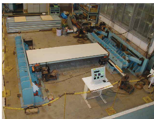
写真3 耐力壁の面内せん断試験の様子 Scene of in-plane shearing test with bearing wall
