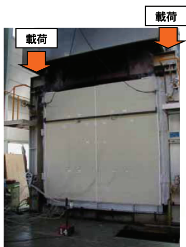
写真4 外壁耐火性能試験の外観 Scene of fire-resistive performance test with exterior wall
