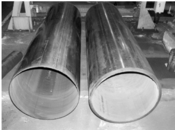
Left: 609.6mm × 6.0mm (24" × 0.24") t/D = 1.0%, Right: 609.6mm × 22.0mm (24" × 0.87") t/D = 3.6%
