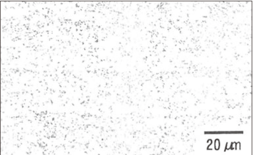
(b) Annealing structure (Ferrite + spheroidal cementite)
