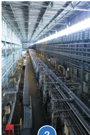
2 Annealing furnace (Horizontal radiant tube furnace)
