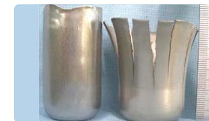
NSSC FW™2 SUS304 (Single cold rolling) Blank dia: \phi 80 mm, Lubricant: JW#122 Punch dia (mm): 1st \phi 40 \rightarrow 2 nd \phi 35 \rightarrow 3 rd \phi 30 \rightarrow 4 th \phi 25
