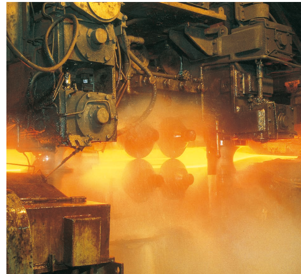
Forming and welding machine for hot electric resistance welding
