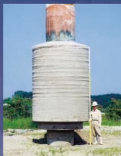
The diameter can be expanded to double the pile size.
