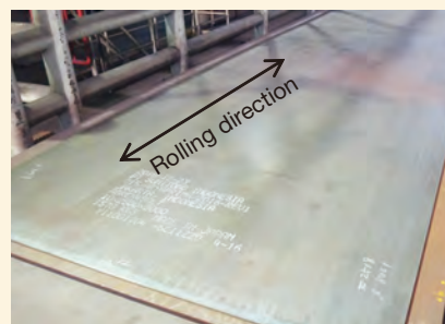
The rolling direction with respect to the stencil markings
