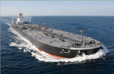
Ship name: TSURUGA Completion: Oct. 2009 Length: 333 m Breadth: : 60 m Dead weight: 300,000 DWT
