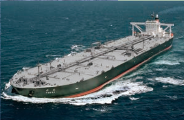
Ship name: TAMBA Completion: Jan. 2009 Length: 333 m Breadth: : 60 m Dead weight: 300,000 DWT
