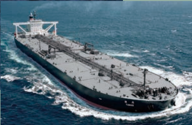
Ship name: TANGO Completion: Oct. 2009 Length: 333 m Breadth: : 60 m Dead weight: 300,000 DWT
