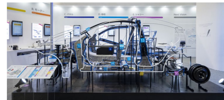
Next-generation automobile's structural concept, "NSafe™-AutoCocept"
