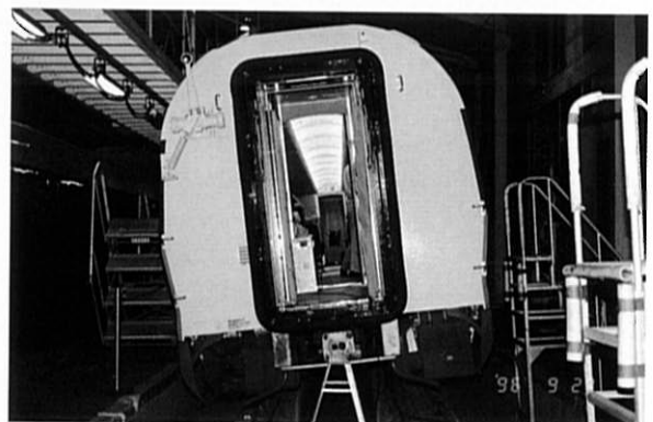
Photo 4 7 degrees tilting carbody on a control test
