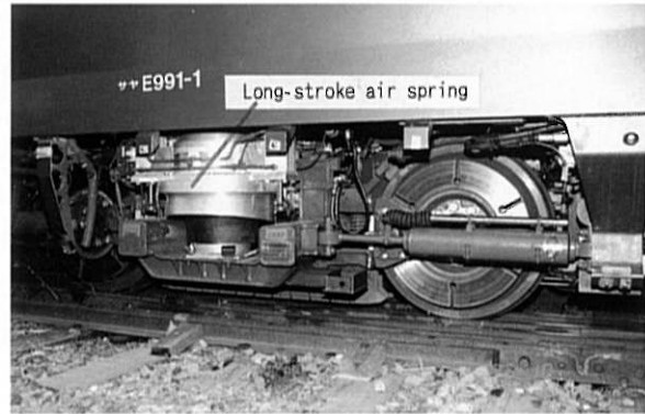
Photo 1 Long-stroke air spring mounted on a bogie
