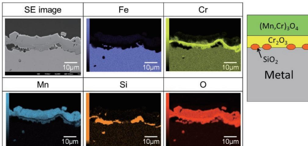
**Fig. 1** Sectional distributions of component elements by SEM/EDX on the surface scale of UNS 32101 heated in normal atmosphere (1200°C, 1 h)<sup>4)</sup>
