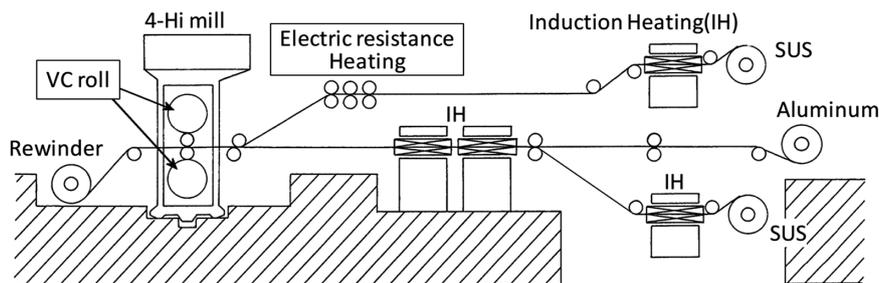
Fig. 5 Outline of clad coil production line<sup>7)</sup>
