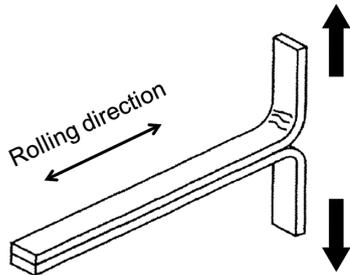
Fig. 6 Shape of test piece for peel test
