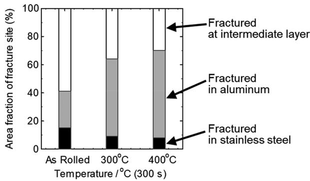
Fig. 9 Relationship between area fraction of fracture site at peel test and heat treatment temperature<sup>10)</sup>
