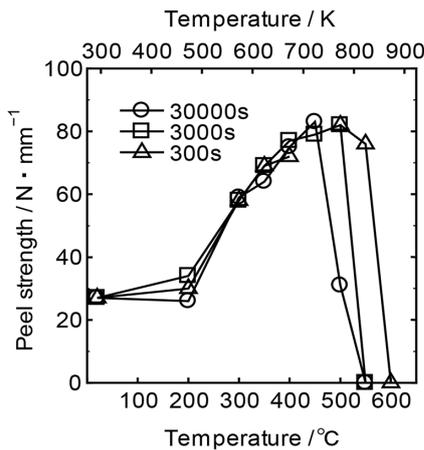
Fig. 7 Effect of heat treatment conditions on peel strength<sup>9)</sup>
