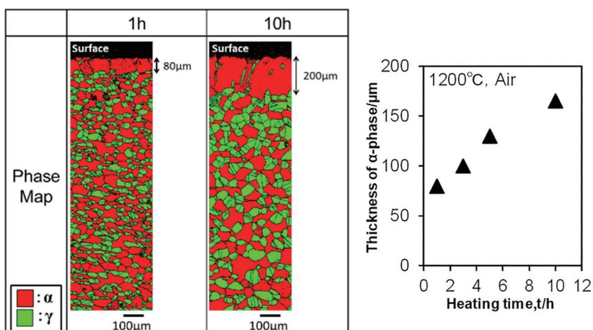
Fig. 2 Phase distribution of UNS 32101 heated in normal atmosphere at 1200°C and thickness change of surface layer in  $\alpha$  phase<sup>4)</sup>
