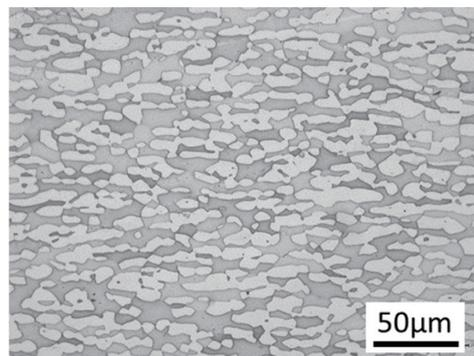
Fig. 3 Typical microstructure of NAR-2120 shaped steel (cross section perpendicular to R.D.)
