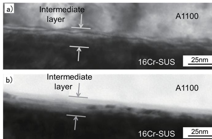
Fig. 8 TEM micrographs of bonding interface: a) as rolled, b) heat treated at 400°C for 300 s<sup>9)</sup>
