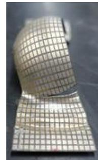
Fig. 6 Broken part of SUS316 (L30×T90 mm)
