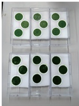
Fig. 6 Photograph of the substrate surface cultures Algae are cultured on glass filters placed on sponges filled with a culture medium in plastic cases. Upper: three-day cultures supplied with air. Lower: three-day cultures supplied with 1%CO 2 .
