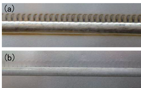
Fig. 10 Appearance of weld bead after electrolytic polishing (a) Before polishing (b) After polishing
