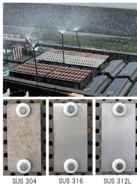
Fig. 3 Seawater shower exposure test 2)
