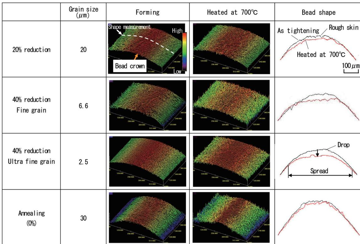
Fig. 12 Bead head shape before and after heated at 700°C for 120 h
