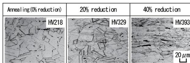
Fig. 7 Metallographic structure and surface hardness of NSSC 302BN with varying rolling ratio
