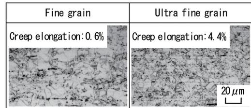
**Fig. 11** Creep test method, creep elongation, and cross-sectional microstructures
