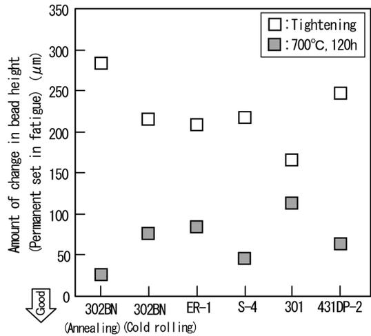
Fig. 4 Measurement results of permanent set amount of each steel
