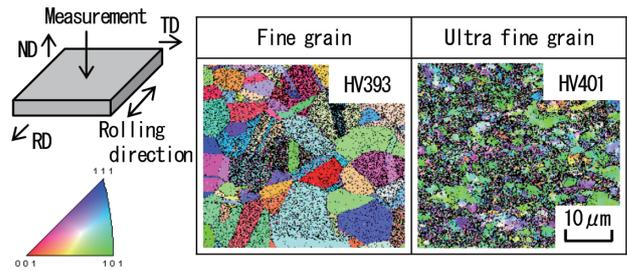
**Fig. 10** Inverse pole figure map (IPF map) and surface hardness of finished rolled material
