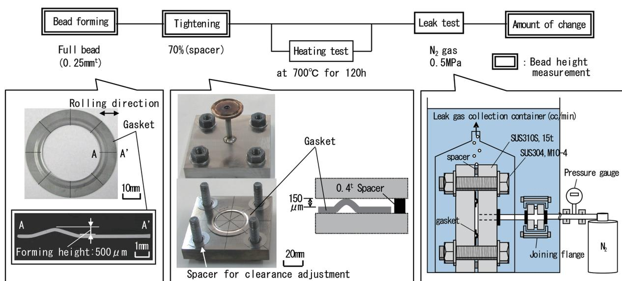
Fig. 2 Evaluation method for gasket properties
