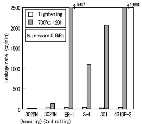
Fig. 5 Measurement results of leakage amount between each process
