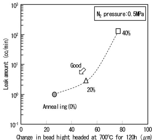
Fig. 8 Relationship between high-temperature permanent set amount after heating at 700°C for 120 h and leak amount
