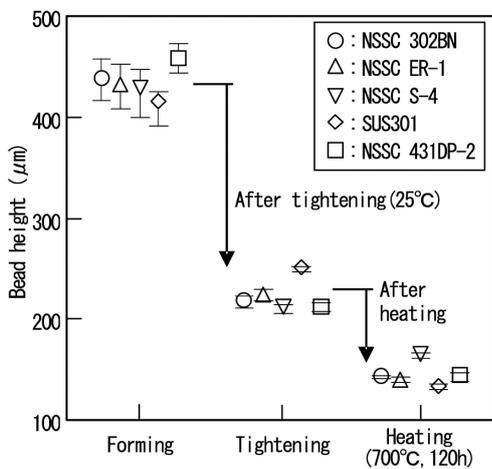
Fig. 3 Height of residual bead after each process
