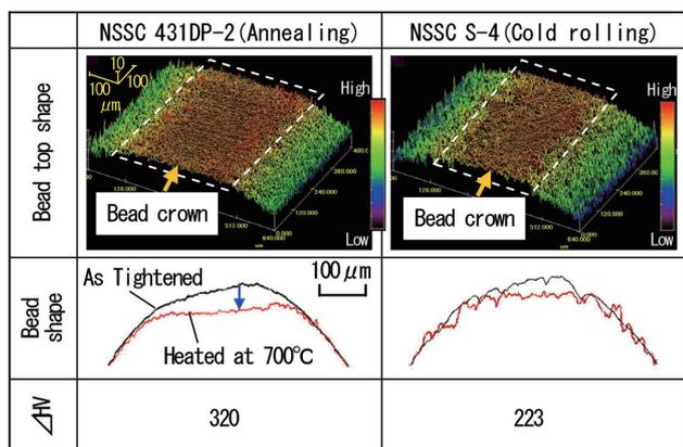
Fig. 6 Bead head shape after heated at 700°C (ΔHV: material hardness-hardness after heating)
