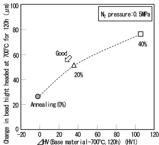
Fig. 9 Relationship between ΔHV after heating at 700°C for 120 h and high-temperature permanent set amount
