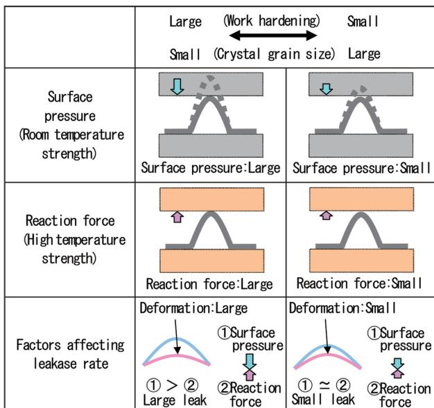
Fig. 13 Schematic of surface pressure and reaction force in 700°C heating evaluation
