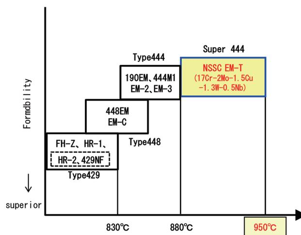
Fig. 1 Heat resistance of different types of stainless steel
