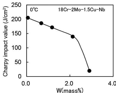
Fig. 6 Effect of W on Charpy impact value of 18Cr-2Mo-1.5Cu-Nb steel
