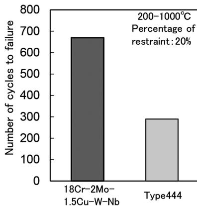
Fig. 8 Thermal fatigue life of round bar test pieces
