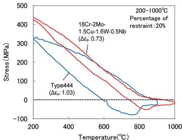
Fig. 7 Temperature-stress curves at tenth cycle of thermal fatigue test
