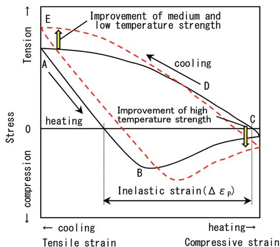
Fig. 2 Schematic diagram of stress-strain curve in thermal fatigue test
