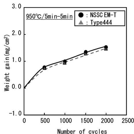
Fig. 12 Cyclic oxidation test of NSSC EM-T
