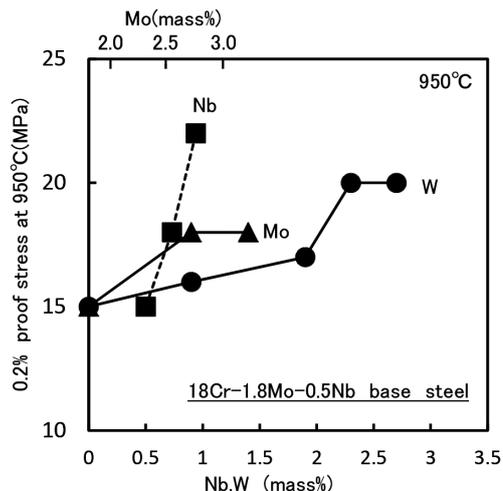
Fig. 5 Effects of Nb, Mo and W on 0.2% proof stress at 950°C
