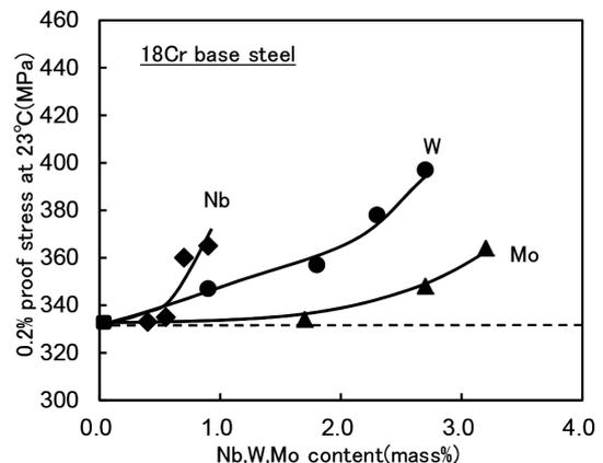
Fig. 3 Effect of Nb, W and Mo on 0.2% proof stress at room temperature
