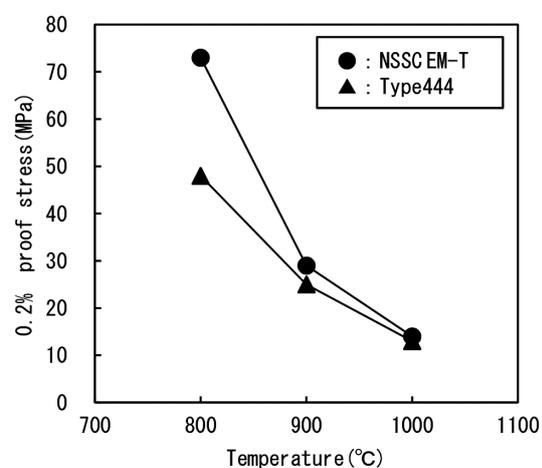
Fig. 9 Tensile properties at elevated temperatures of NSSC EM-T and Type444
