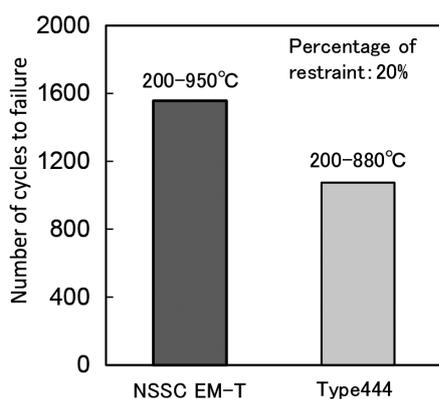
Fig. 10 Thermal fatigue life of ERW pipes of NSSC EM-T
