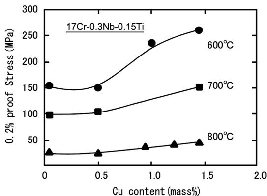
Fig. 4 Effect of Cu on 0.2% proof stress at 600, 700 and 800°C<sup>3)</sup>
