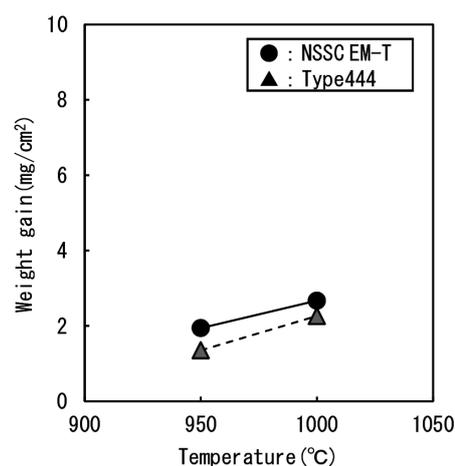
Fig. 11 Continuous oxidation test of NSSC EM-T
