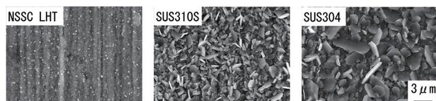
Fig. 6 SEM images of surface after heat treatment at 800°C for 1 hour in air
