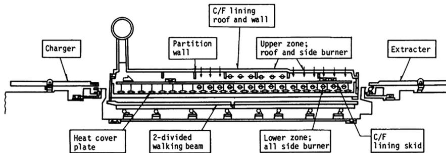
Fig. 2 Schematic diagram of East Nippon Works Kimitsu plate No. 4 heating furnace
