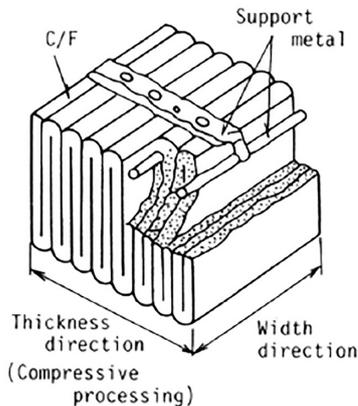
Fig. 3 Ceramic fiber block (Z-BLOK)
