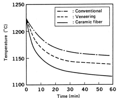
Fig. 4 Comparison of thermal inertia refractories
