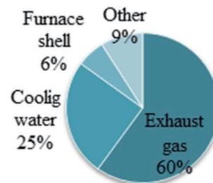
Fig. 10 Thermal energy loss ratio of Kyushu Works Oita hot strip continuous furnace
