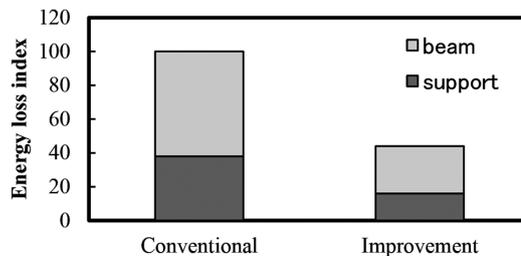
Fig. 14 Calculation of energy loss index through skid-beam/support lining
