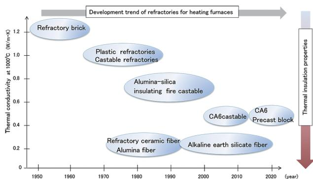
Fig. 1 Development trend and thermal insulation performance of refractories for heating furnaces
