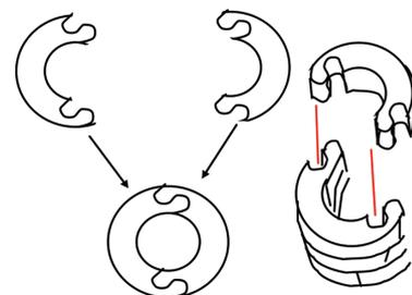
Fig. 8 Schematic figure of new joint combination structure
