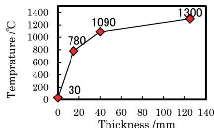
Fig. 12 Inner temperature of the improved lining for a skid-support
