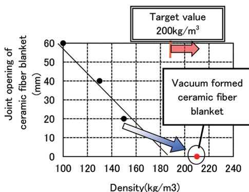
Fig. 7 Relationship between joint opening of ceramic fiber blanket and their density
