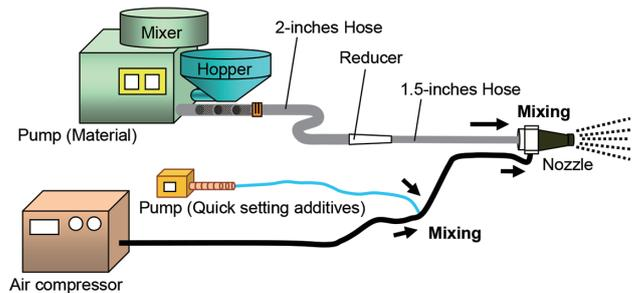
Fig. 9 Schematic diagram of CA6 insulating castable gunning system
