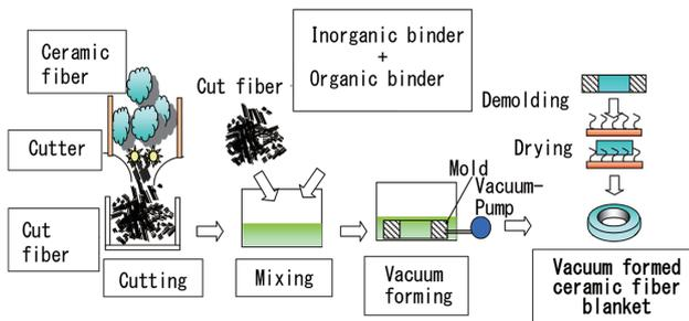
Fig. 6 Making method of Vacuum form
