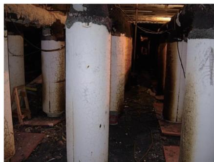
Photo 4 Skid-supports after 5 years in the furnace of the hot-strip mill
