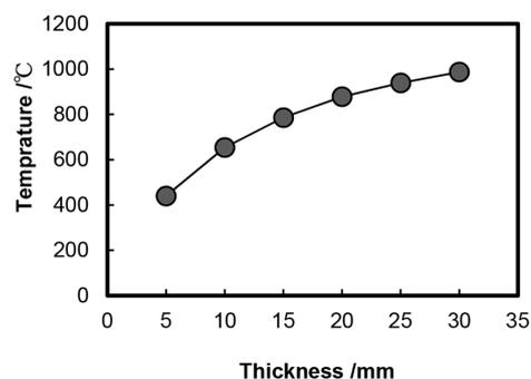
Fig. 13 Calculation of the relationship between the thickness of the high-insulation panel and the surface temperature
