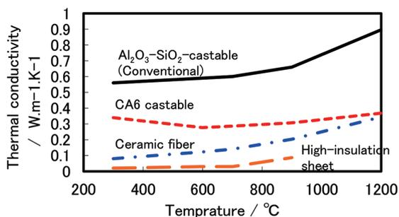
Fig. 11 Thermal conductivity of refractories
