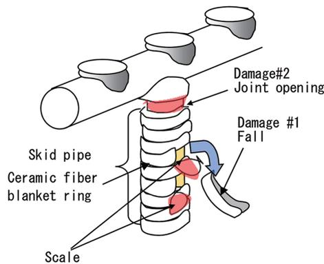
Fig. 5 Damage of the ceramic fiber blanket ring caused by scale
