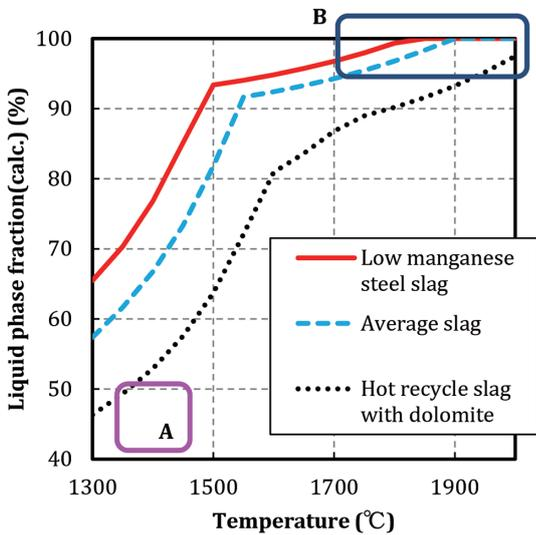
Fig. 19 Calculated liquid phase fraction of slag
