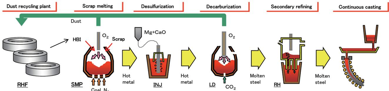
Fig. 1 Steel manufacturing process at Hirohata Works
