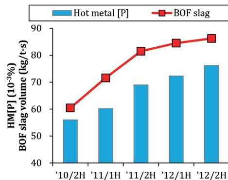
Fig. 3 Relation between hot metal [P] and BOF slag volume
