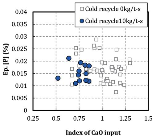
Fig. 11 Influence of slag cold recycle on [P] at blowing end point
