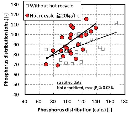
Fig. 8 Influence of slag hot recycle on (P)/[P] ratio
