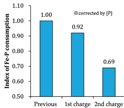
Fig. 25 Influence of all slag hot recycle on consumption of phosphorus alloy
