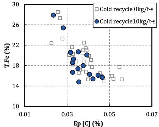
Fig. 14 Relation between blowing end point carbon and iron content in slag
