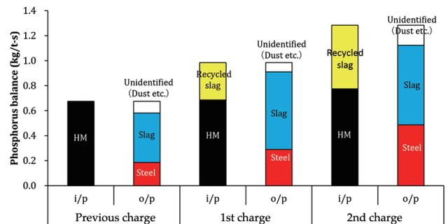
Fig. 24 Mass balance of phosphorus during all slag hot recycle operation
