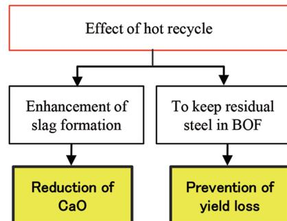
Fig. 10 Effect of slag hot recycle
