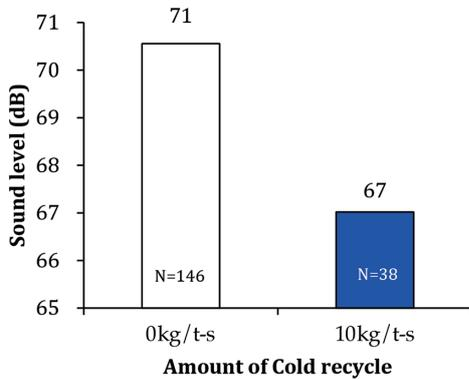
Fig. 15 Influence of slag cold recycle on sound level
