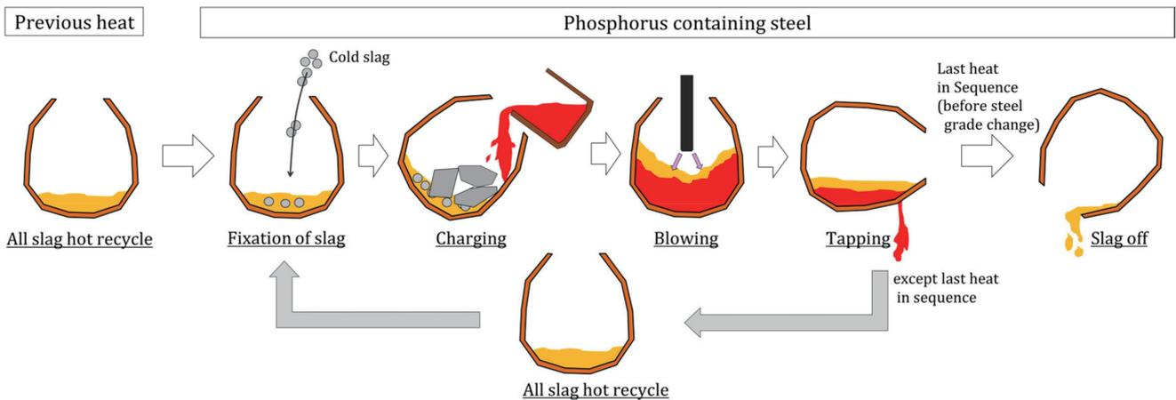
Fig. 21 Schematic view of all slag hot recycle operation
