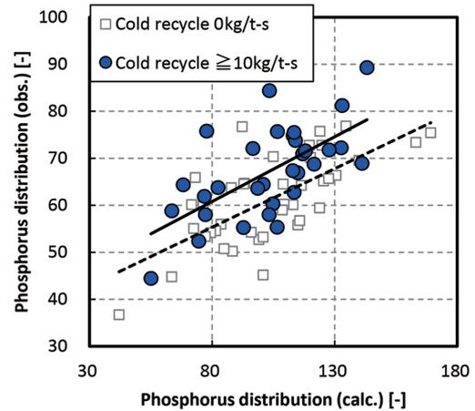
Fig. 13 Influence of slag cold recycle on (P)/[P] ratio
