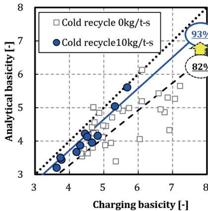
Fig. 12 Relation between charging basicity and analytical basicity
