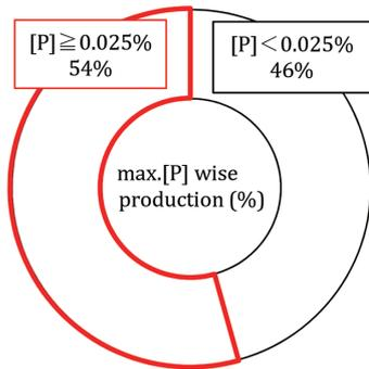
Fig. 5 Production structure of phosphorus containing steel
