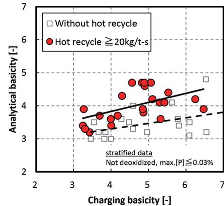
Fig. 9 Relation between charging basicity and analytical basicity
