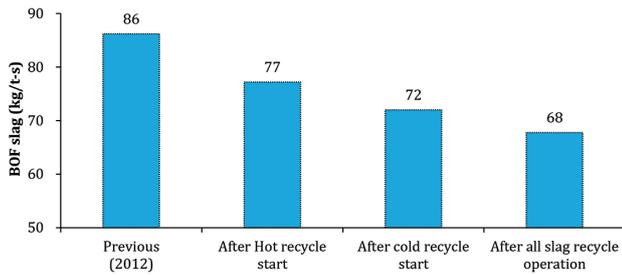
**Fig. 26 Improvement of BOF slag generation by development of slag recycle operation**
