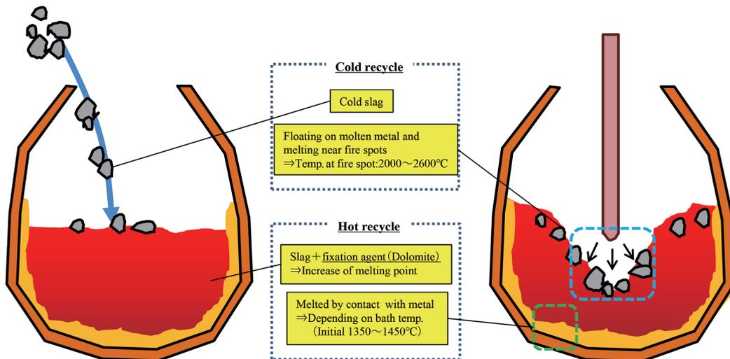
Fig. 20 Schematic view of melting phenomena of recycled slag
