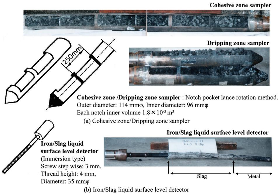
Fig. 11 State of collected samples by samplers and liquid level detector
