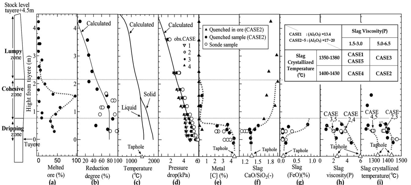
Fig. 14 Vertical distribution of sample analysis results by dissection and sampling sonde (eleventh test operation)
