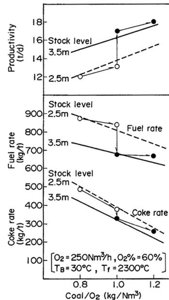
Fig. 7 Comparison of operation results of oxygen injection and calculation results
