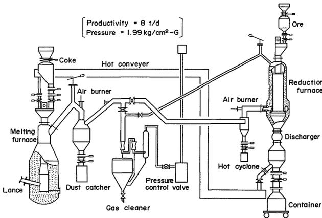
Fig. 5 Schematic diagram of the SC pilot plant
