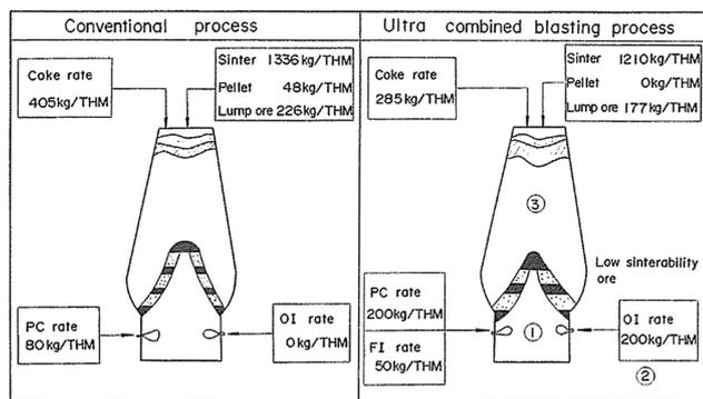
Fig. 15 Concept of ultra combined blasting for blast furnace
