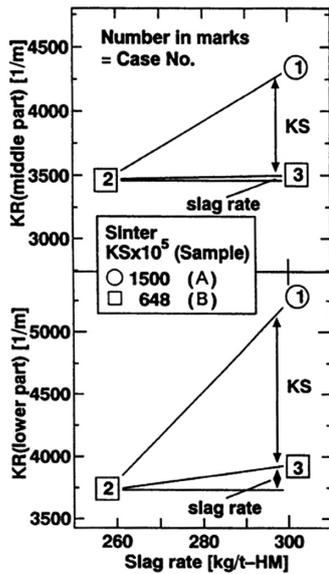
Fig. 18 Comparison of effect of KS on KR with that of slag rate
