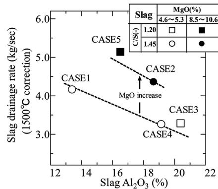
Fig. 20 Effect of the slag content on drainage rate
