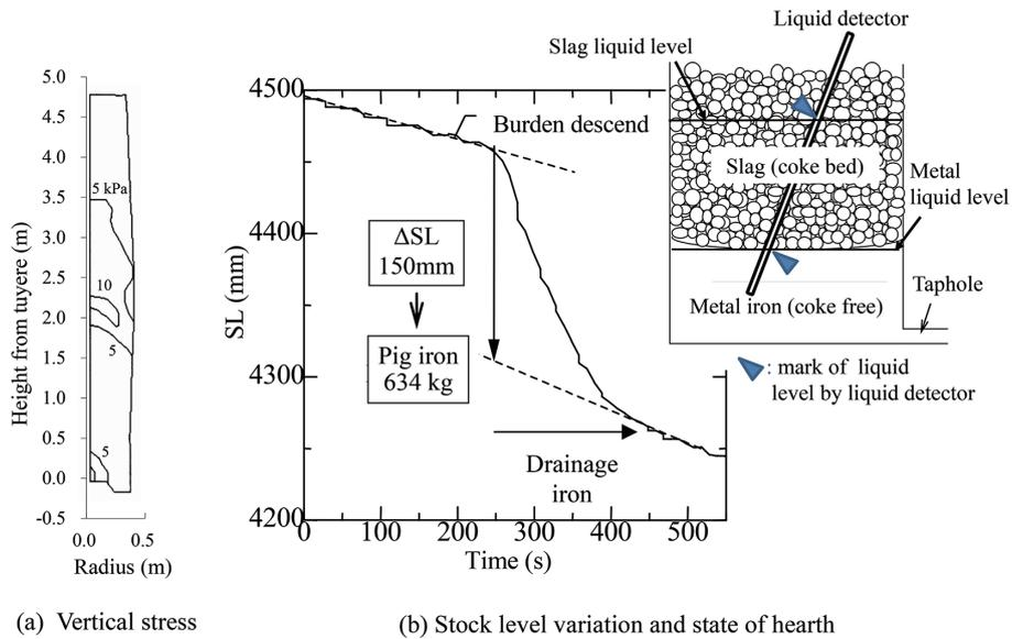
Fig. 12 Vertical stress, variation of stock level with drainage and state of hearth (eleventh test operation)
