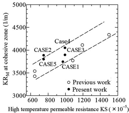
Fig. 22 Effect of sinter high temperature property  $KS$  on permeable resistance index of cohesive zone  $KR_M$  of experimental blast furnace
