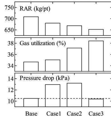
Fig. 26 Influence of layer structure on reducing agent rate, gas utilization and pressure drop
