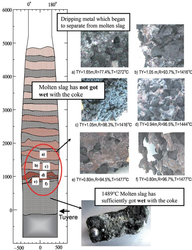
Fig. 13 Dissection of experimental blast furnace (thirteenth test operation)
