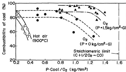
Fig. 2 Results of the coal combustion test
