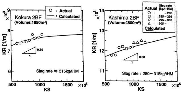
Fig. 19 Effect of KS on KR in the commercial blast furnace
