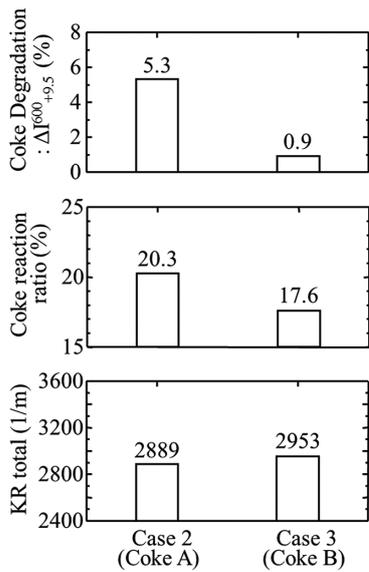
Fig. 24 Comparison of effect of CRI on coke degradation, reaction ratio and KR
