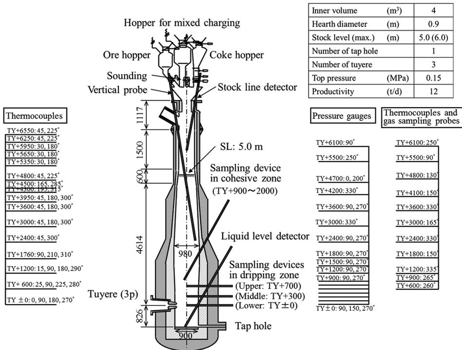
Fig. 10 Schematic diagram of the experimental blast furnace
