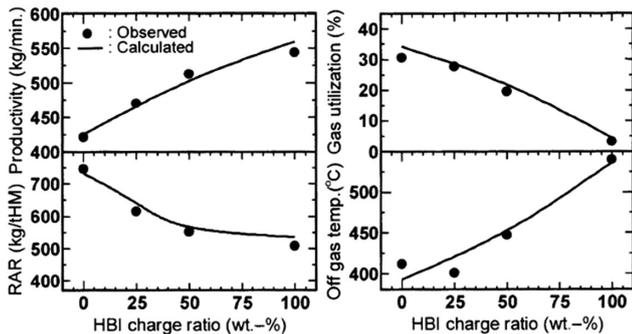
Fig. 17 Calculated results of experimental blast furnace operation
