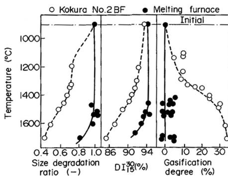
Fig. 6 Distributions of coke properties and gasification degree in melting furnace
