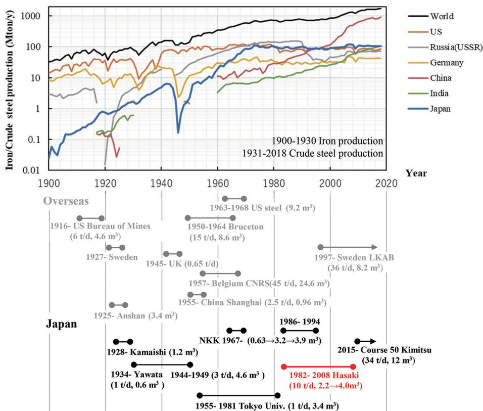
Fig. 1 Transitions of iron and crude steel production and experimental blast furnaces
