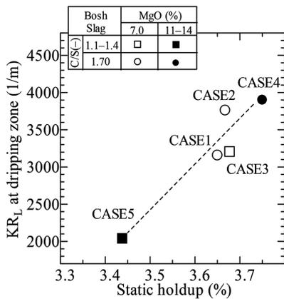
Fig. 21 Effect of calculated static hold-up on permeable resistance index of dripping zone  $KR_L$  of experimental blast furnace
