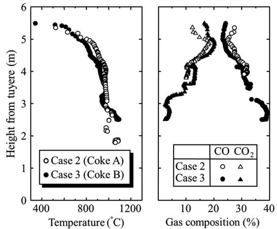
Fig. 23 Vertical distribution of temperature and gas composition
