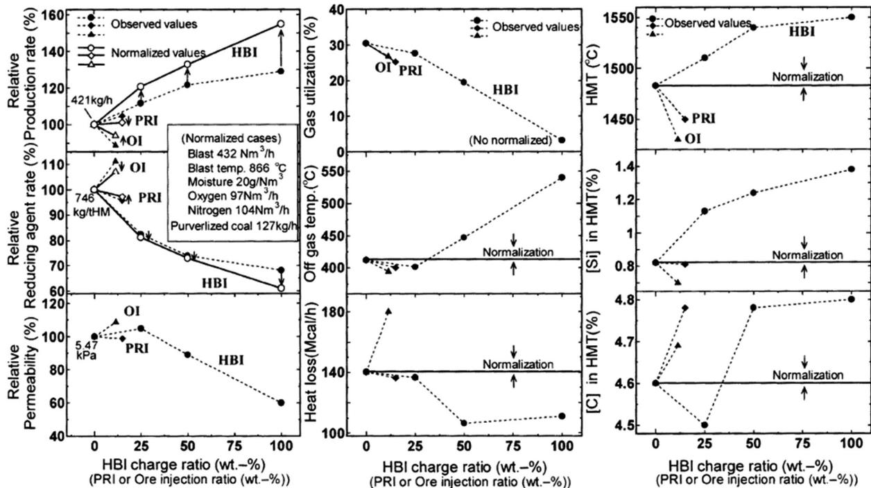
Fig. 16 Relative production rate, reducing agent rate and permeability through the reduced iron melting tests using experimental blast furnace
