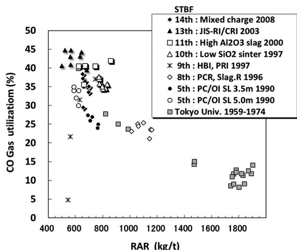
Fig. 27 Relationship between reducing agent rate and gas utilization of experimental blast furnaces
