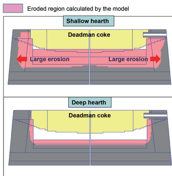
Fig. 24 Effect of hearth depth on erosion of hearth refractories
