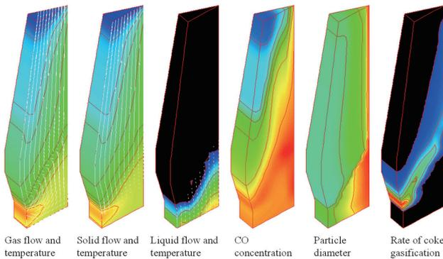
Fig. 4 In-furnace states calculated with the 3D dynamic simulator for blast furnace
