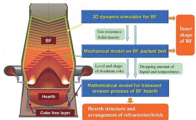
Fig. 17 Technologies of design for blast furnace with combining mathematical blast furnace models
