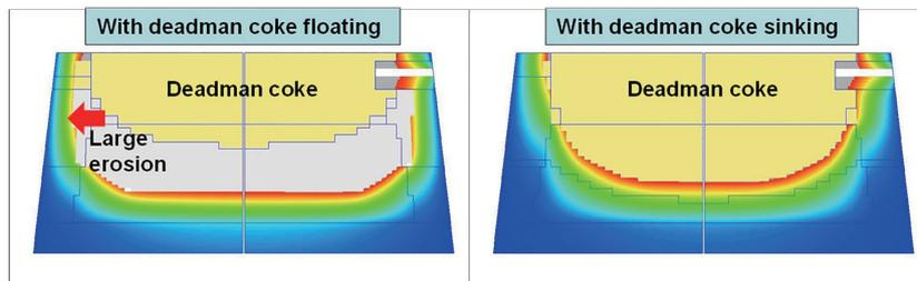
Fig. 14 Influence of deadman coke level in hearth on erosion of hearth refractories
