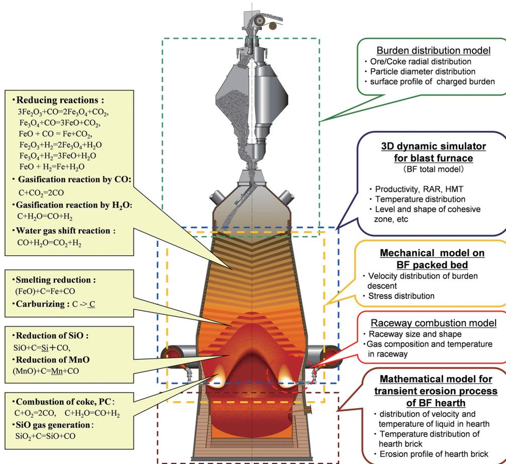
Fig. 2 Phenomena in blast furnace and mathematical models
