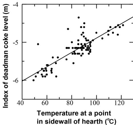
Fig. 15 Relation between index of deadman coke level and temperature of sidewall of hearth
