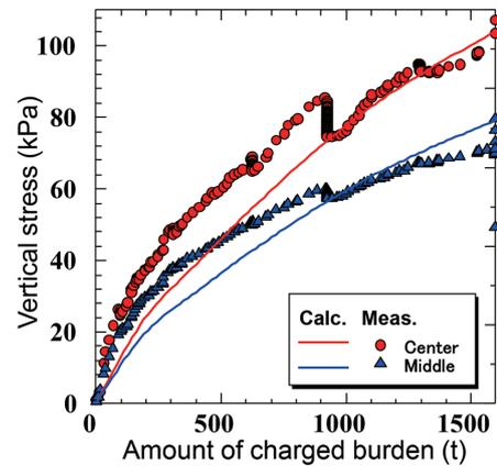
Fig. 10 Comparison of calculated vertical stress by the mechanical model on BF packed bed with measured one during filling raw materials in Kokura 2BF
