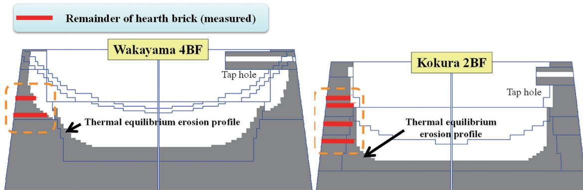
Fig. 13 Comparison of erosion profile of hearth between calculated results by the mathematical model for transient erosion process of BF and measured ones
