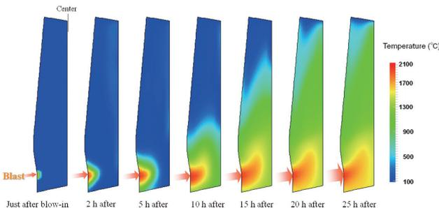
Fig. 5 Transition of solid temperature in a blast furnace after blow-in calculated with the 3D dynamic simulator for blast furnace
