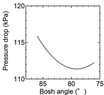
Fig. 23 Relation between bosh angle and pressure drop
