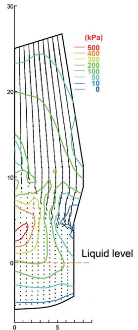
Fig. 12 Sinking level and its shape calculated by the mechanical model on BF packed bed
