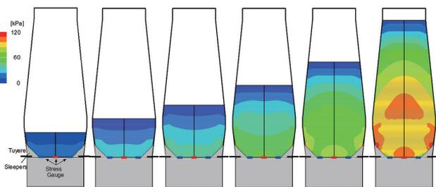
Fig. 9 Vertical stress distribution calculated by the mechanical model on BF packed bed during filling raw materials in Kokura 2BF
