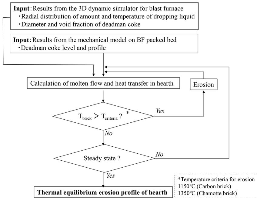
Fig. 11 Flowchart of the mathematical model for transient erosion process of blast furnace hearth
