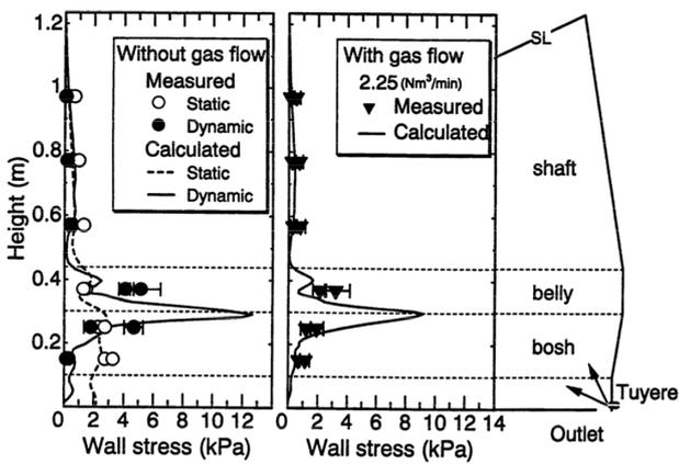
Fig. 7 Comparison of normal stresses on the wall between calculated results by the mechanical model on BF packed bed and measured results (1/20 cold model experiment)
