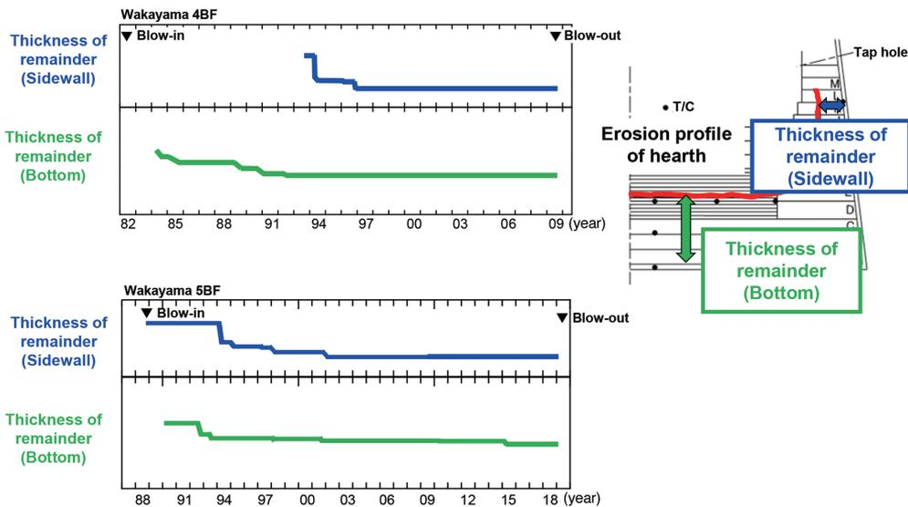
Fig. 16 Transition of maximum erosion of hearth refractories estimated by measured temperature of hearth in Wakayama 4BF and 5BF
