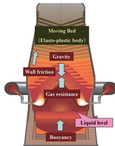
Fig. 6 Forces acting on moving bed in a blast furnace
