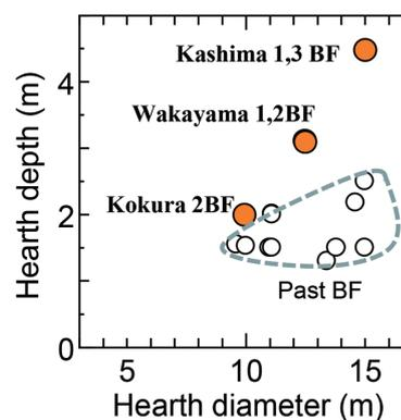
Fig. 25 Relation between hearth diameter and hearth depth of blast furnace in Wakayama, Kokura and Kashima
