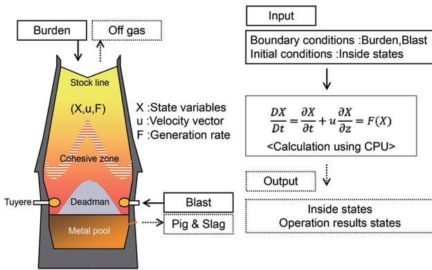
Fig. 3 Outline of 3D dynamic simulator for blast furnace
