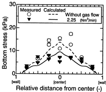
Fig. 8 Comparison of normal stresses on the bottom between calculated results by the mechanical model on BF packed bed and measured results (1/20 cold model experiment)
