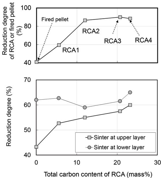
**Fig. 5** Influence of carbon content of RCA on reduction degree of materials at 1100°C
