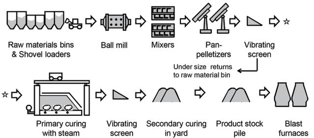
**Fig. 15 Production flow sheet of RCA implemented in Oita Works**
