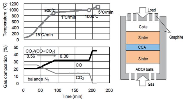
Fig. 1 Tests procedure of reduction test under load
