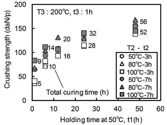
Fig. 11 Influence of holding time at 50°C in the primary curing on crushing strength of RCA
