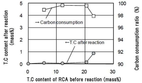
**Fig. 6** Influence of carbon content of RCA on residual carbon after reaction at 1100°C
