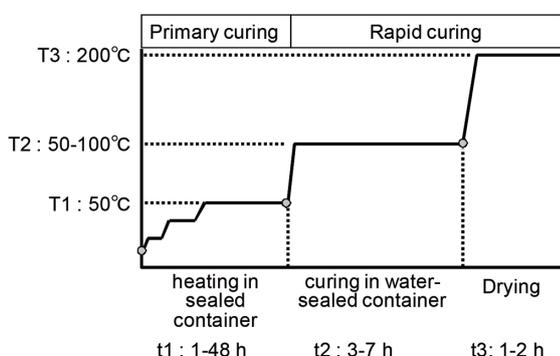
Fig. 3 Conditions and parameters of rapid curing test in small-scale batch
