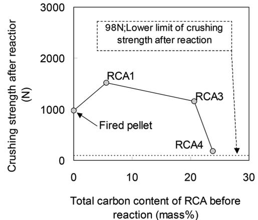
**Fig. 8** Relationship between total carbon in RCA before reaction and crushing strength after reaction
