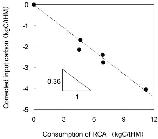
Fig. 10 Relationship between consumption of RCA and corrected input carbon
