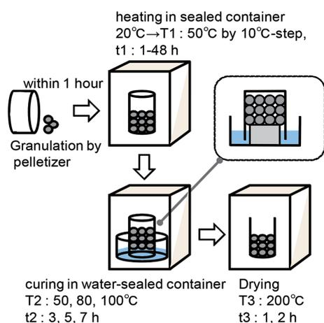
Fig. 2 Batch test procedure of rapid curing of RCA
