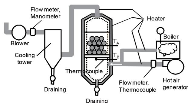
Fig. 4 Schematic diagram of continuous rapid curing test
