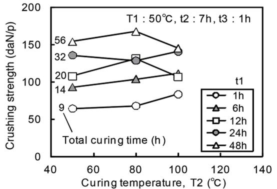
Fig. 12 Influences of holding time at high temperatures t2 (A) and curing temperature T2 (B) on crushing strength
