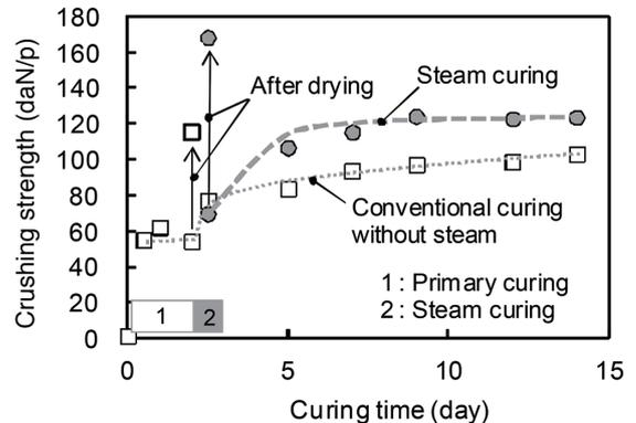
**Fig. 14 Curing behavior of RCA after steam curing for 12 hours**
