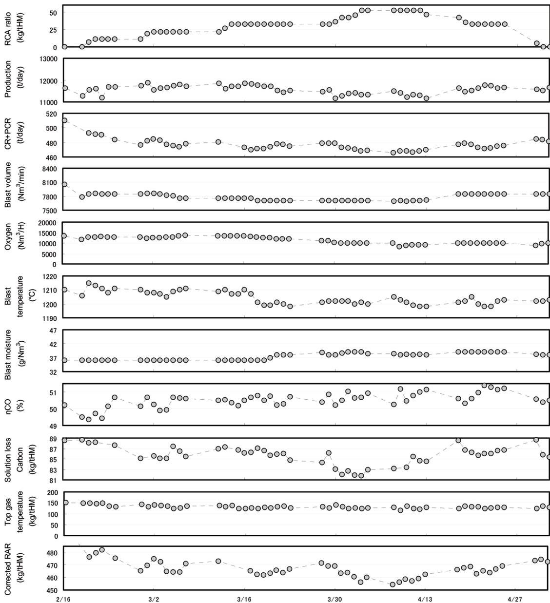
Fig. 9 Operational results of plant trial test of RCA at Oita No. 2 BF
