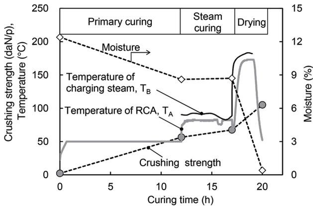
**Fig. 13 Results of continuous curing test**
