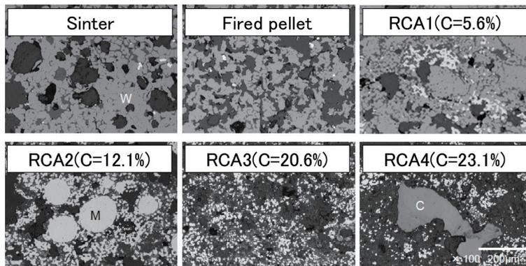
**Fig. 7** Microstructure of carbon composite agglomerate after reduction at temperature up to 1100°C, together with sinter and fired pellet
