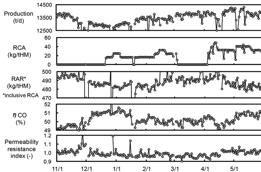
Fig. 16 Operational data of RCA use in Oita No. 1 Blast Furnace
