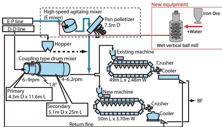
Fig. 12 Granulation process of the Wakayama No.5 Sinter Machine
