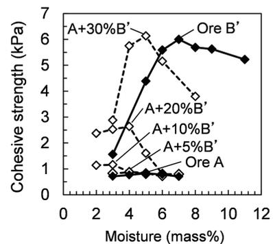
**Fig. 7 Cohesive strength of sample ores**
