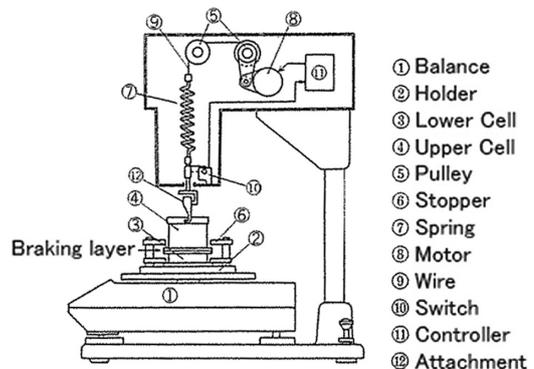
**Fig. 6 Schematic diagram of cohesive strength tester<sup>12)</sup>**
