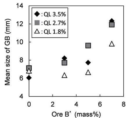
**Fig. 9 Effect of micro-particle binder on granulation at E-P line<sup>9)</sup>**
