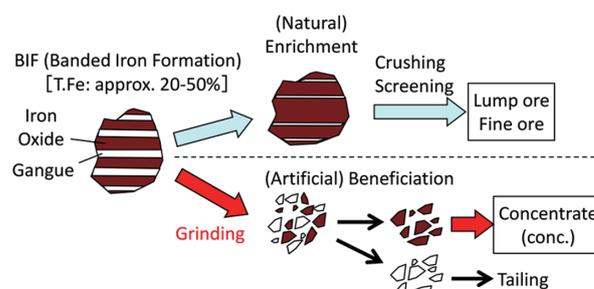
Fig. 1 Schematic diagram of beneficiation process
