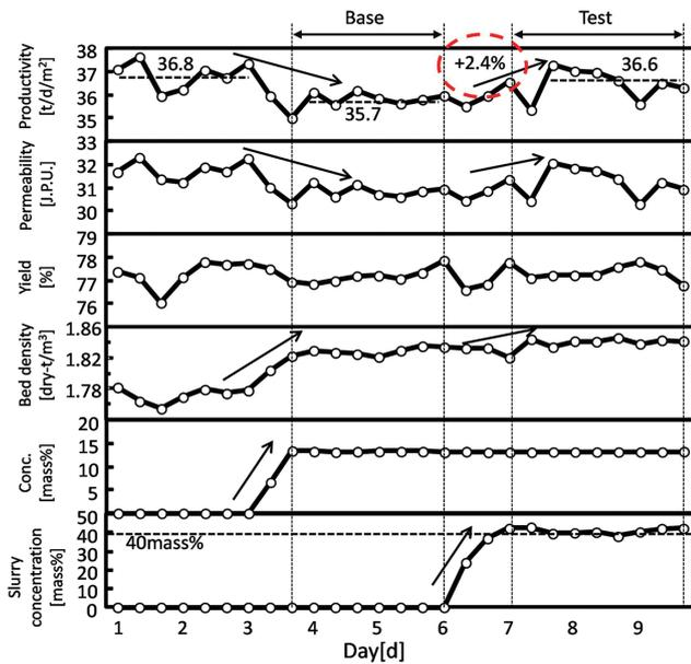
Fig. 17 Effect of micro-particle binder addition on sintering operation at the Wakayama No.5 Sinter Machine<sup>10)</sup>
