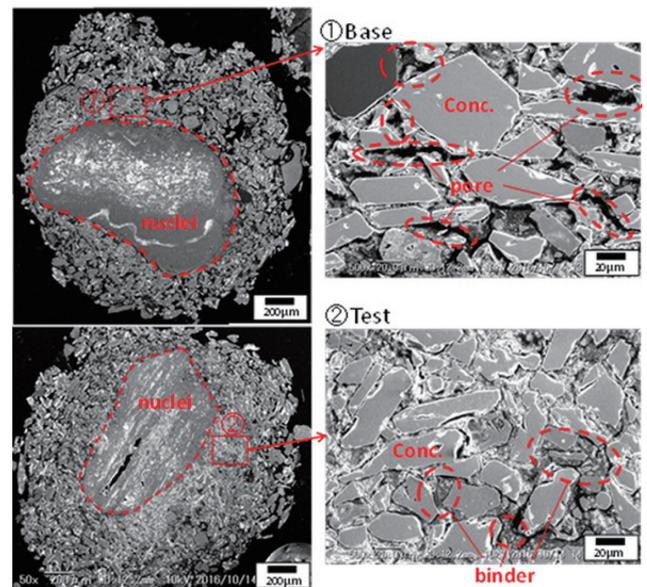
Fig. 16 Effect of micro-particle binder on adhering layer structure
