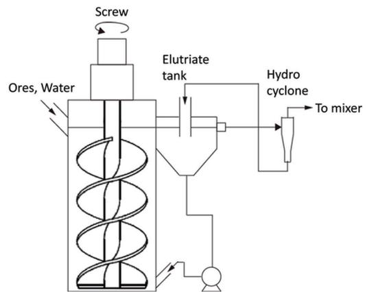
Fig. 13 Schematic diagram of wet vertical ball mill
