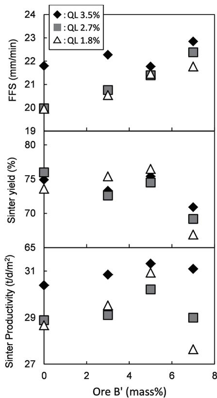
Fig. 11 Effect of micro-particle binder on sinter productivity
