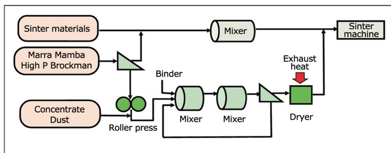
Fig. 3 Process flow of SPEXII<sup>4)</sup>
