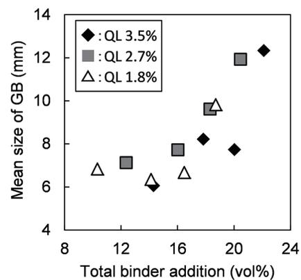
**Fig. 10 Effect of total binder on granulation at E-P line<sup>9)</sup>**
