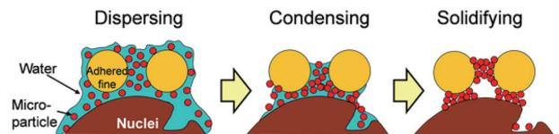
Fig. 2 Behavior of micro-particle on granulation<sup>7)</sup>
