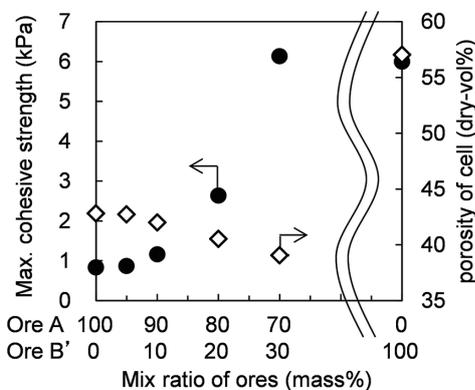
Fig. 8 Changing of maximum cohesive strength by adding micro-particles
