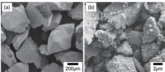
**Fig. 5 SEM image of samples (a) Ore A, (b) Ore B'**
