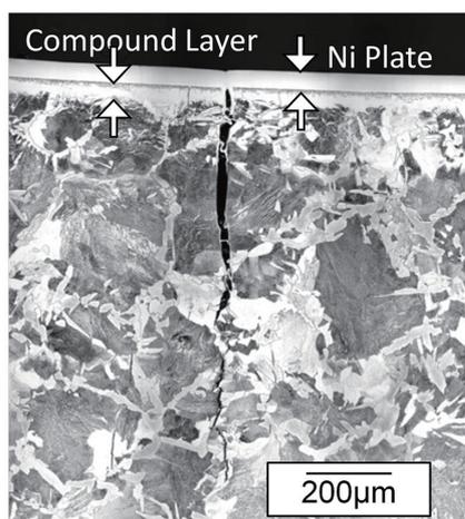
Fig. 1 Image of a crack introduced by bending at the surface of nitrocarburized steel
