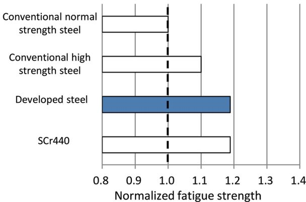
Fig. 5 Normalized fatigue strength of developed steel and conventional steels (Fatigue strength of conventional normal strength steel is taken as 1.0)
