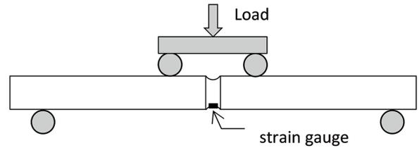
Fig. 6 Schematic of four-point bending test
