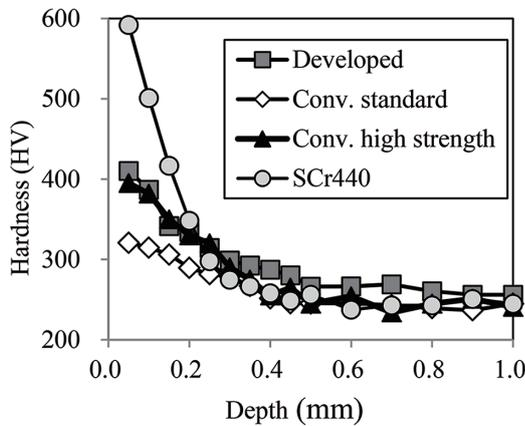
Fig. 4 Hardness profiles of nitrocarburized layers of various steels
