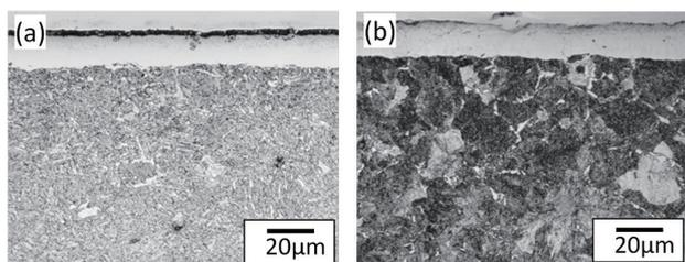
Fig. 8 Images of the cross sections of the nitrocarburized layers in (a) Developed steel and (b) S50C
