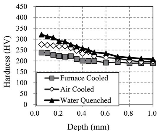
Fig. 10 Effect of the cooling rate at the cooling following re-heating on the hardness profiles of nitrocarburized S40C
