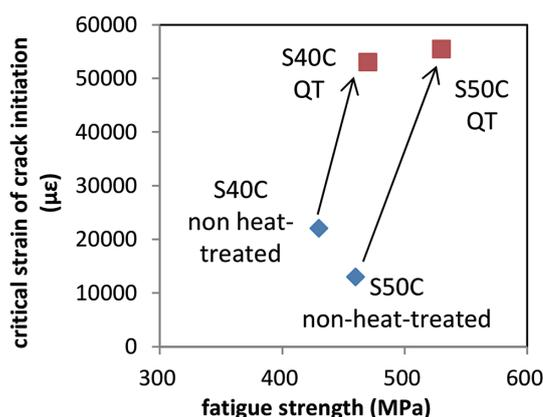
Fig. 2 Effect of quench-and-tempering on fatigue strength and critical strain of crack initiation in the nitrocarburized carbon steel
