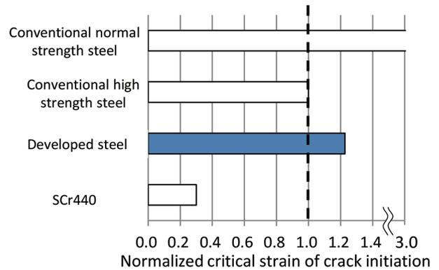
Fig. 7 Normalized critical crack initiating strain of developed steel and conventional steels (Critical strain of conventional high strength steel is taken as 1.0)
