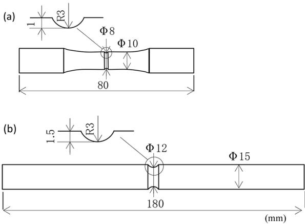
Fig. 3 Shapes of specimens for (a) Rotary bending fatigue test and (b) Four-point bending test
