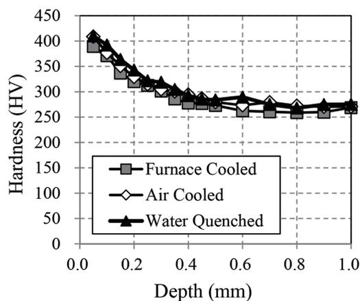
Fig. 11 Effect of the cooling rate at the cooling following re-heating on the hardness profiles of the nitrocarburized developed steel
