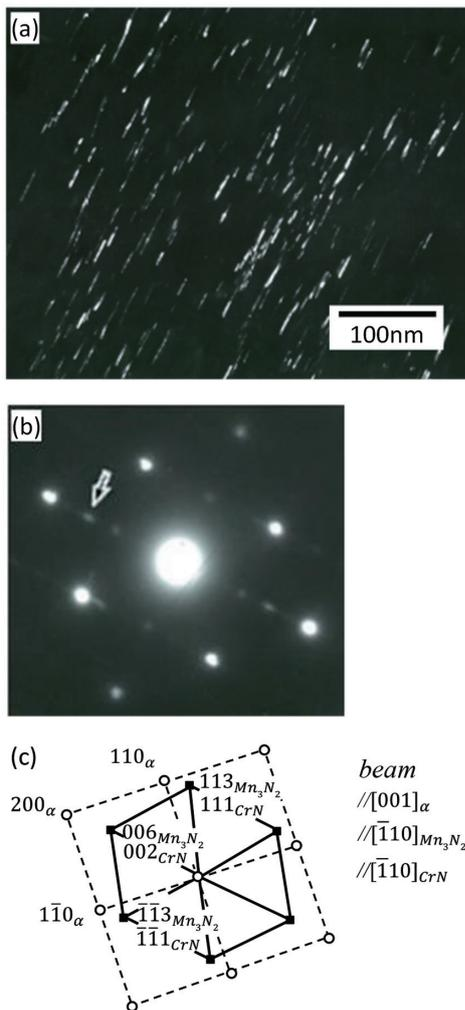
Fig. 12 TEM image taken at a depth of 75  $\mu\text{m}$  below the surface of the diffusion layer in the developed steel (a) Dark field image, (b) Selected area diffraction pattern, and (c) Corresponding key diagram to (b).
