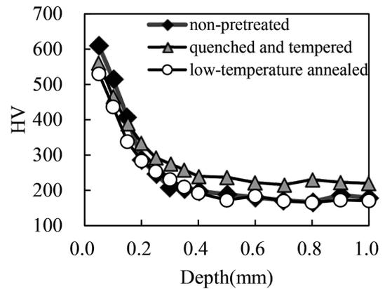
Fig. 8 Effects of quenching-and-tempering and low-temperature annealing followed by nitrocarburizing on hardness profiles of the diffusion layers in SCr420
