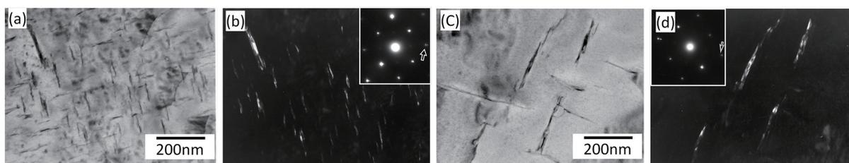
**Fig. 4** TEM images taken in diffusion layer of the nitrocarburized S40C
