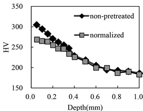
Fig. 2 Effect of normalizing followed by nitrocarburizing on a hardness profile of the diffusion layers (S40C)
