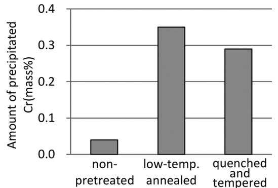
Fig. 9 Effects of the pre-heat treatments on amount of Cr precipitated as a part of cementite
