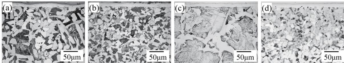
Fig. 1 Optical micrographs of the cross sections of the nitrocarburized surface in (a) Non-pretreated S40C, (b) S40C normalized at 1373 K, (c) Non-pretreated SCr420 and (d) SCr420 normalized at 1123 K
