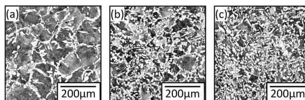
**Fig. 10** Optical micrographs of cross sections of the core matrix (a) Forged at 1523 K, (b) Forged at 1413 K, (c) Forged at 1293 K
