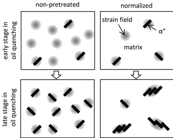
Fig. 6 Schematics of behavior of  $\alpha''$  precipitation during oil quenching in the non-pretreated specimen and the normalized specimen
