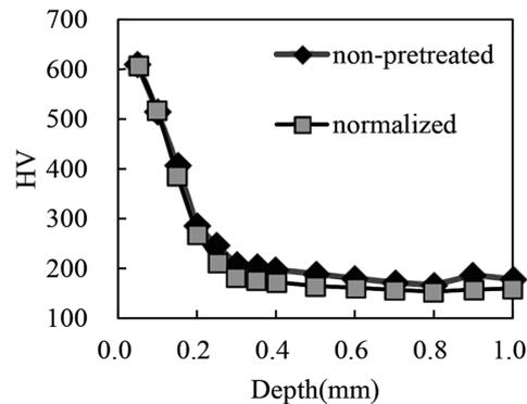
Fig. 3 Effect of normalizing followed by nitrocarburizing on a hardness profile of the diffusion layer (SCr420)
