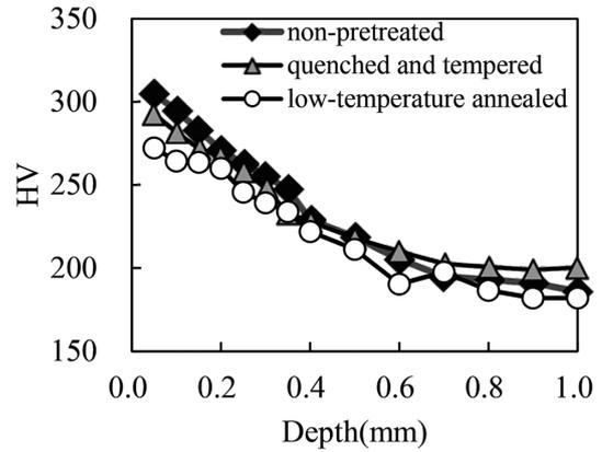
Fig. 7 Effects of quenching-and-tempering and low-temperature annealing followed by nitrocarburizing on hardness profiles of the diffusion layers in S40C
