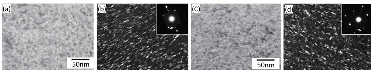
**Fig. 5** TEM images taken in diffusion layer of the nitrocarburized SCr420
