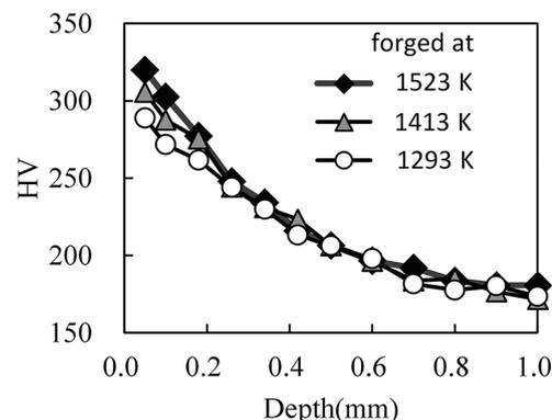
**Fig. 11** Effect of forging temperature on hardness profiles of the diffusion layers
