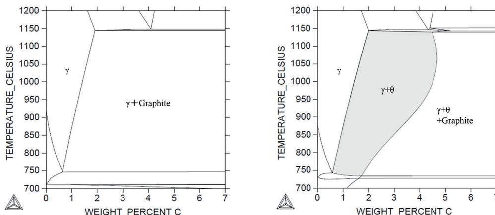
Fig. 9 Equilibrium phase diagrams of Fe-C system, a) MSB20 and b) SCM420
