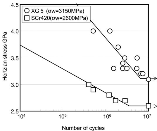
Fig. 5 Results of roller pitting fatigue test with XG5
