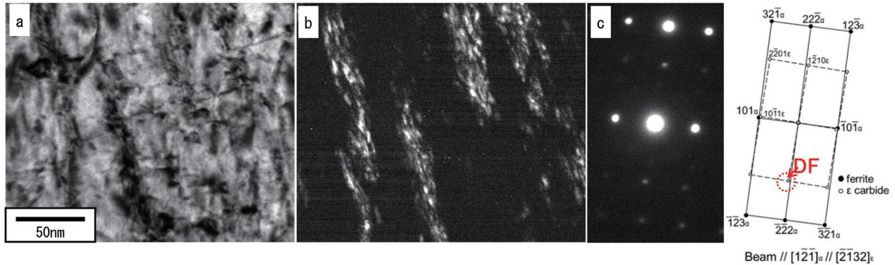
Fig. 4 TEM images of 0.6C-1Si steel tempered 400°C, a) Bright field image, b) Dark field image, c) Selected area diffraction pattern
