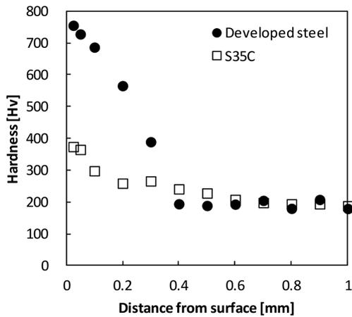
Fig. 11 Hardness profile of nitrided layers of developed steel and S35C
