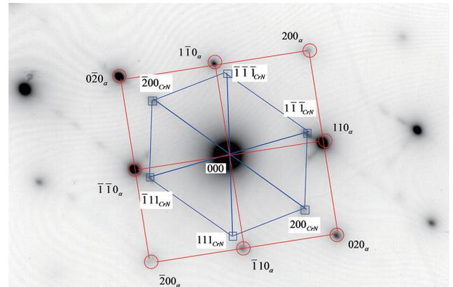
Fig. 13 Selected area diffraction pattern taken in nitrided developed steel and corresponding key diagram
