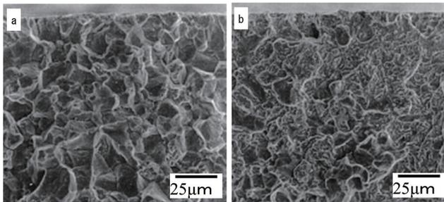
Fig. 8 SEM (scanning electron microscopy) images of impact fatigue fracture origin, a) SCM420: Intergranular fracture, b) B-added: Transgranular fracture
