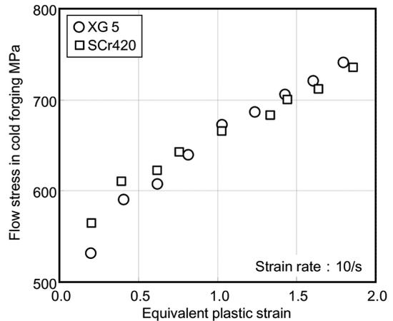
Fig. 6 Flow stress in cold forging in XG5
