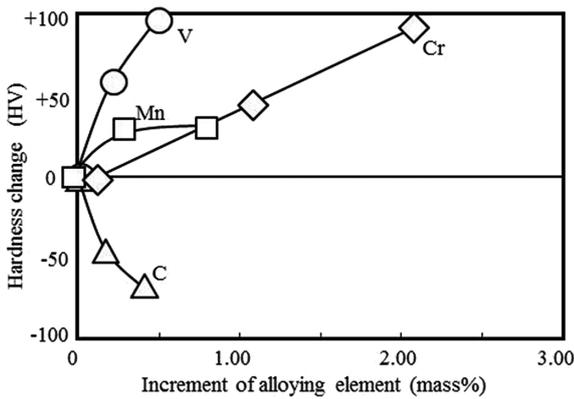
Fig. 10 Effect of alloying element amounts to the nitrided surface hardness
