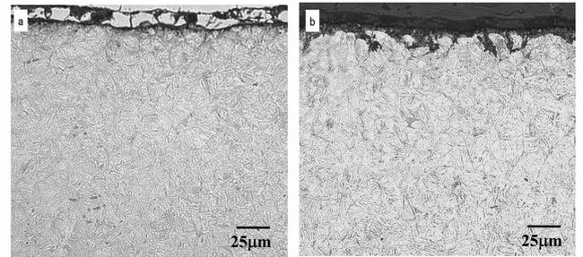
Fig. 2 Micrographs of carburizing layer (nital etching), a) CM201, b) SCM420
