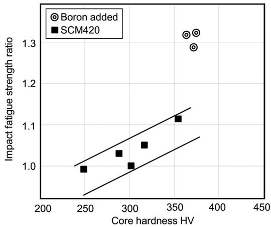
Fig. 7 Results of impact fatigue test
