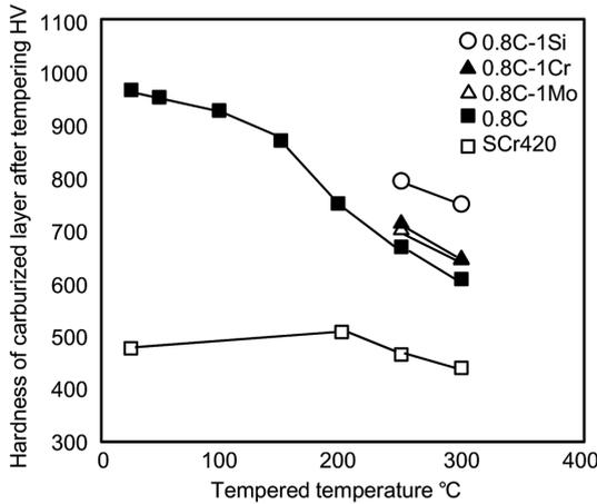
Fig. 3 Hardness of carburized layer after low temperature tempering with varying alloy element contents
