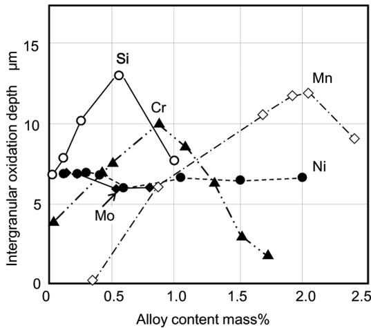
Fig. 1 Intergranular oxidation depths varying alloy contents
