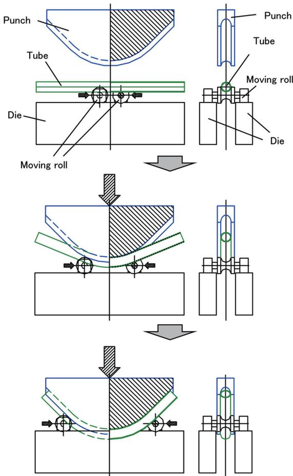
Fig. 5 Forming processes of press bending with moving rolls
