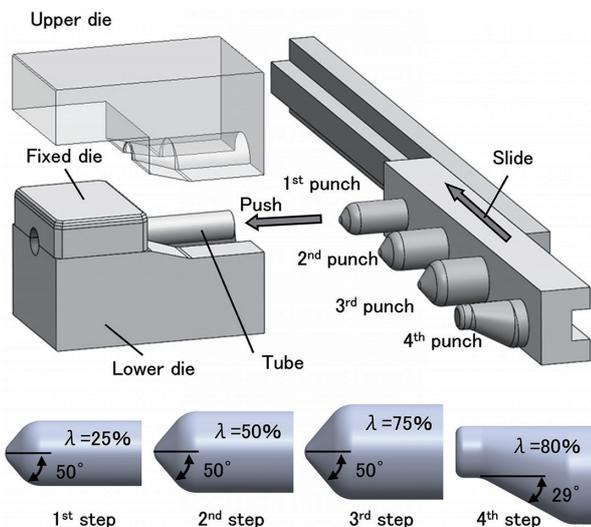
Fig. 21 Punch shape of each step of tube end expanding with eccentricity
