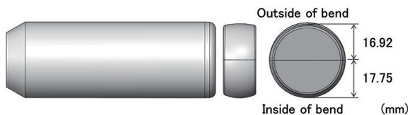
**Fig. 2** Shape of asymmetry mandrel ball
