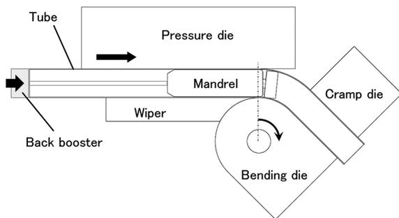
**Fig. 1** Outline of rotary draw bending method
