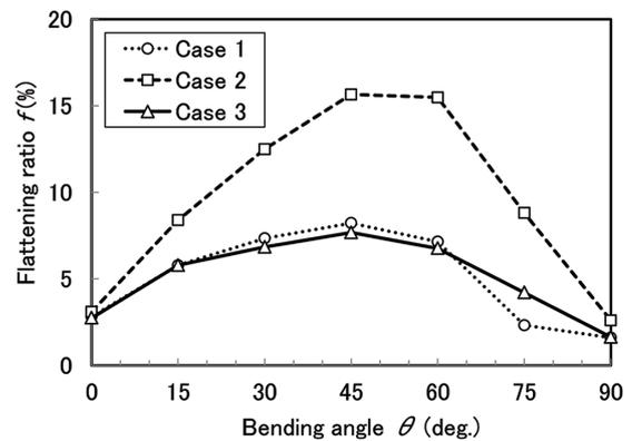
**Fig. 4** Distribution of flattening ratio after rotary draw bending
