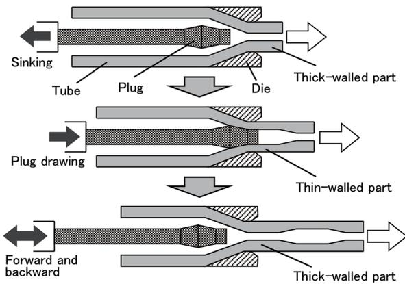
Fig. 24 Forming process of tube with different wall thickness by drawing
