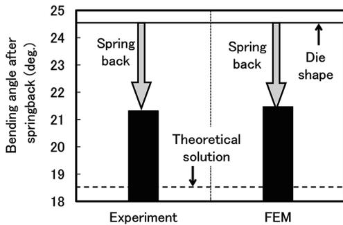
Fig. 11 Springback after press bending with cross-sectional deformation
