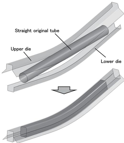
Fig. 9 Outline of press bending with cross-sectional deformation
