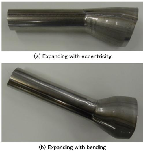
Fig. 23 Mechanical expanding samples with eccentricity or bending
