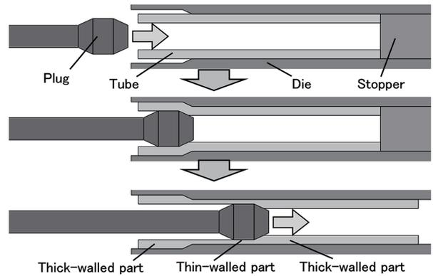
Fig. 26 Forming process of tube with different wall thickness by ironing
