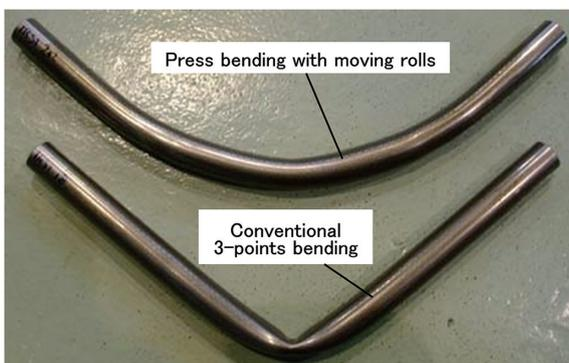
Fig. 6 Comparison of forming shapes between press bending with moving rolls and conventional 3-points bending
