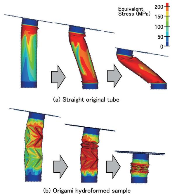
Fig. 19 Comparison of FEM results of axial crushing in case of 10 degrees of impact angle
