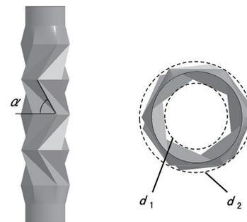
Fig. 20 Design parameters of origami structure
