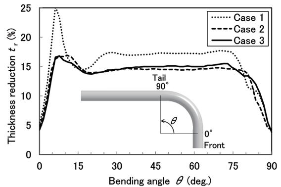
**Fig. 3** Distribution of thickness reduction at tension side after rotary draw bending
