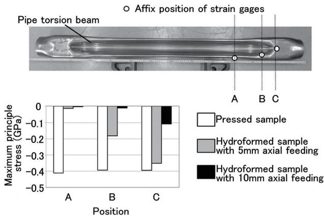
Fig. 16 Residual stress after forming of torsion beam
