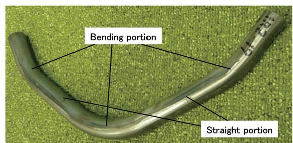
Fig. 7 Sample formed by press bending method with moving rolls to apply to a shape with several bending portions
