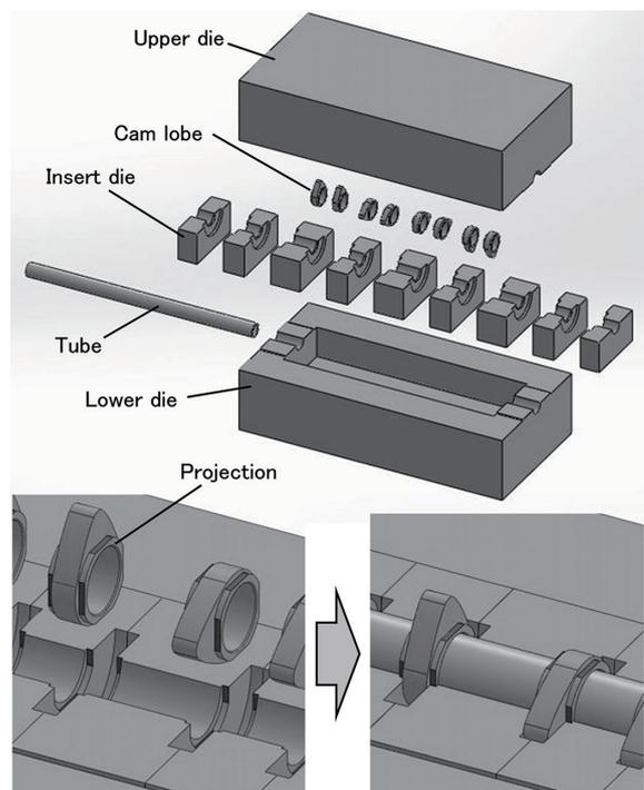
Fig. 14 Hydroforming die structure for high accurate camshaft
