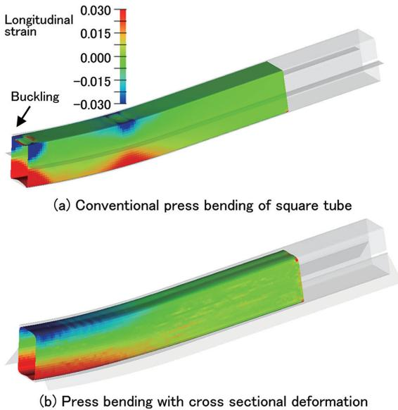
Fig. 10 Comparison of longitudinal strain after press bending
