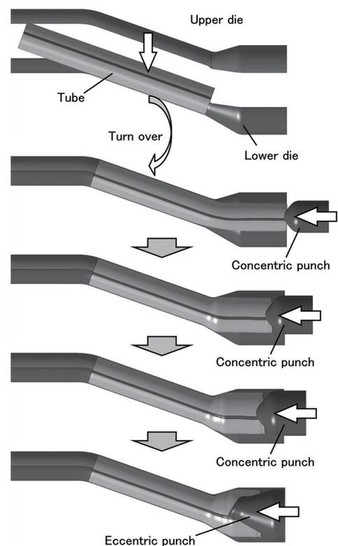
Fig. 22 Forming process of expanding at tube end after press bending
