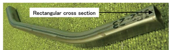
Fig. 8 Sample with rectangular cross section formed by press bending method with moving rolls
