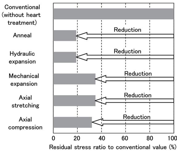
Fig. 17 Comparison of residual stress ratio to conventional value in torsion beam
