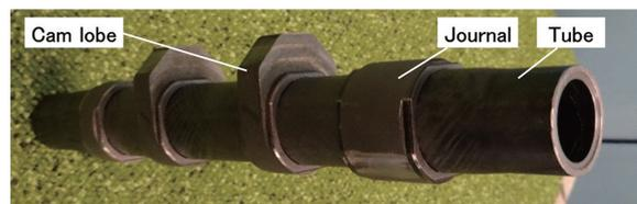
Fig. 15 Simple shape camshaft made with high accurate hydroforming die
