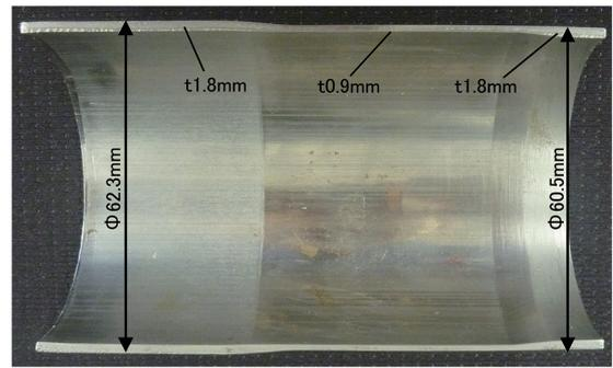
Fig. 27 Forming sample of tube with different wall thickness by ironing
