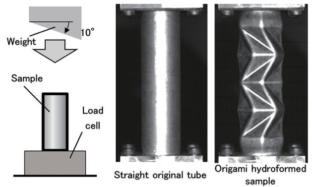
Fig. 18 Impact test procedure
