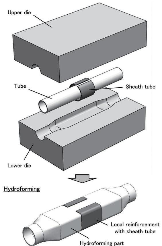
Fig. 12 Local reinforcement by hydroforming with sheath tube
