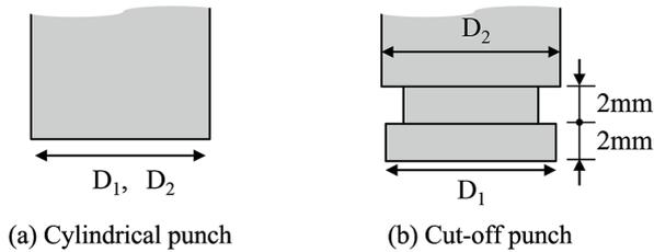
Fig. 3 Schematic figure of piecing tools
