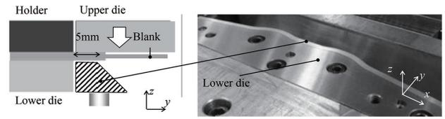
Fig. 10 Developed trimming die structure for suppressing excessive bending behavior around trim edge line
