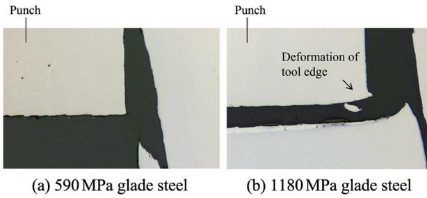
Fig. 12 Deformation of sheared tool edge
