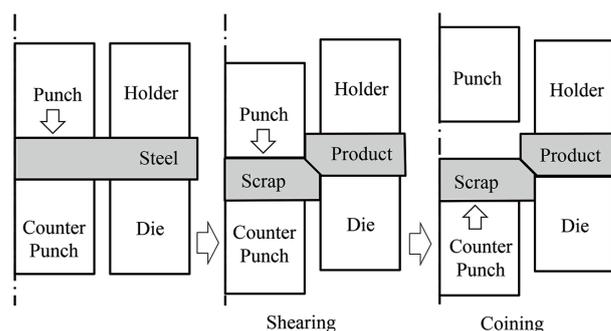
**Fig. 1** Schematic of coining method with aid of scrap
