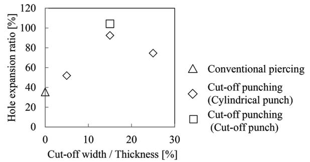
Fig. 5 Hole-expansion ratio of cut-off punched hole
