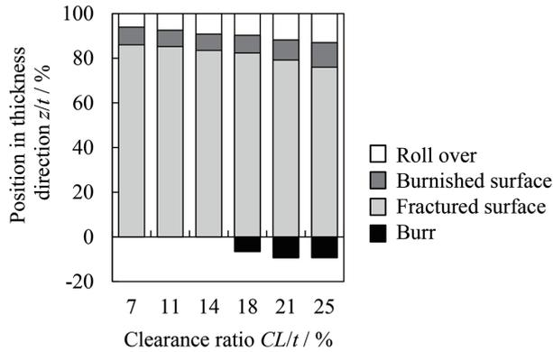
Fig. 8 Effect of piercing clearance on pierced edge quality
