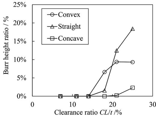
Fig. 9 Comparison of effect of shearing clearance on burr height among different trimming line curvatures
