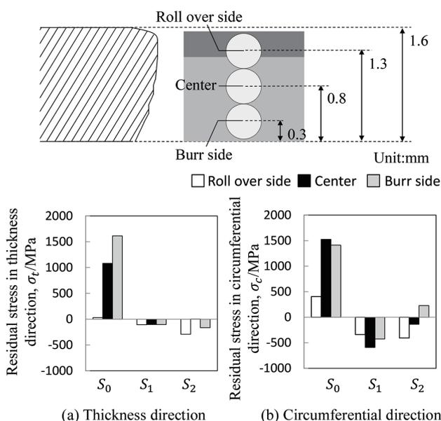
**Fig. 2** Residual stress at each coining stroke
