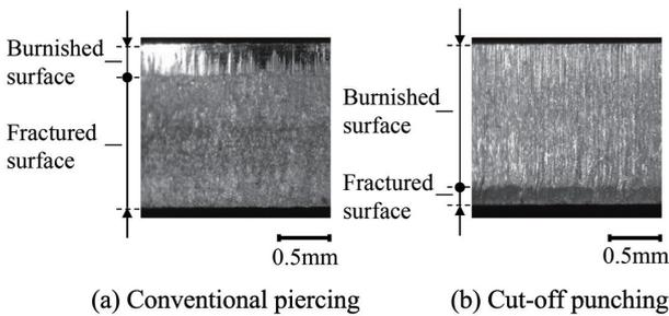
Fig. 4 Sheared surface of conventional piercing and cut-off punching
