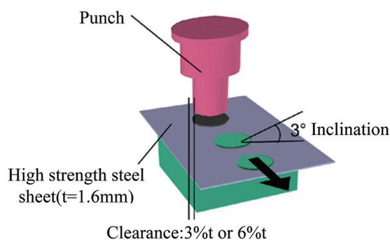
Fig. 14 Schematic diagram of pierce processing test
