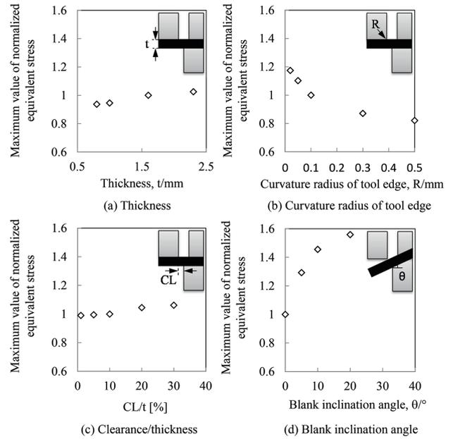
Fig. 13 Influences of shearing conditions on tool edge stress
