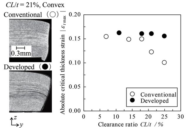
Fig. 11 Effect of developed trimming die structure on flange-up formability
